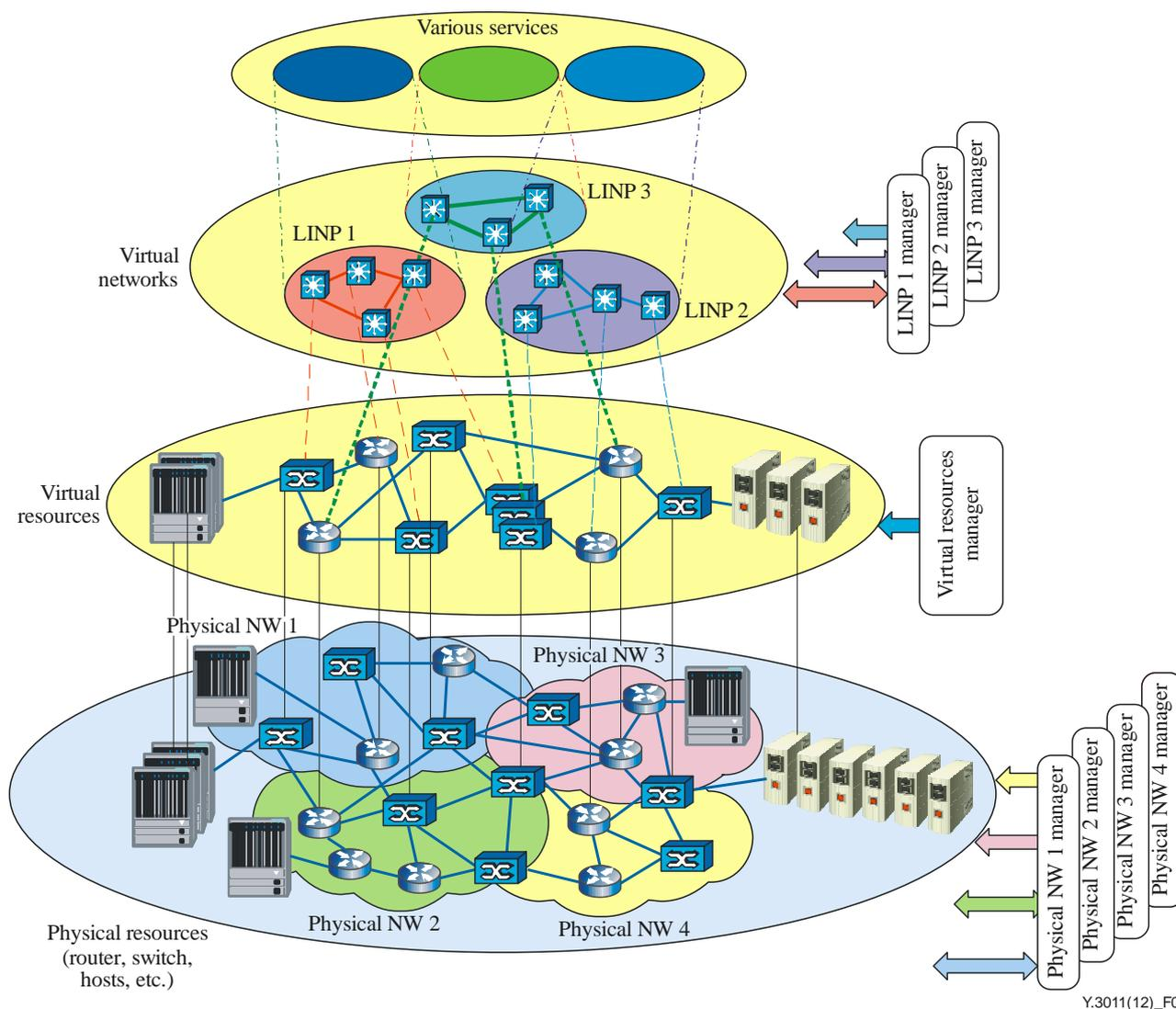
**Figure 1 – Conceptual architecture of network virtualization**
