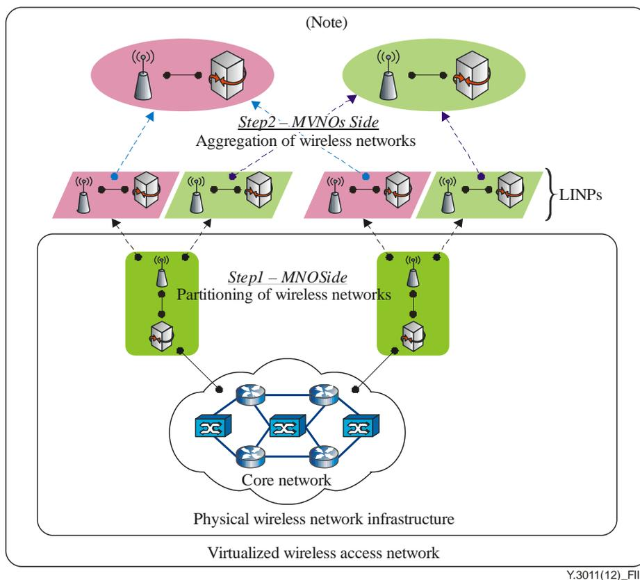
NOTE – Use case 3: Composite use case comprised of partitioning and aggregation of wireless networks
