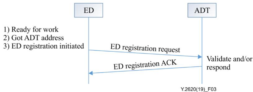
**Figure 3 – ED registration procedure**
