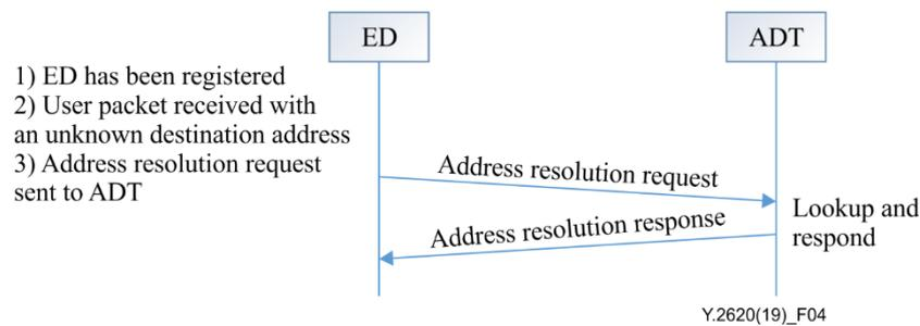
**Figure 4 – Address resolution procedure**
