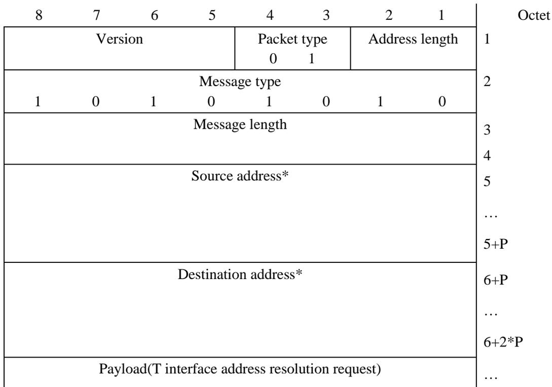
\* NOTE – This field length is determined by the field address length, and represented by P (octets)
