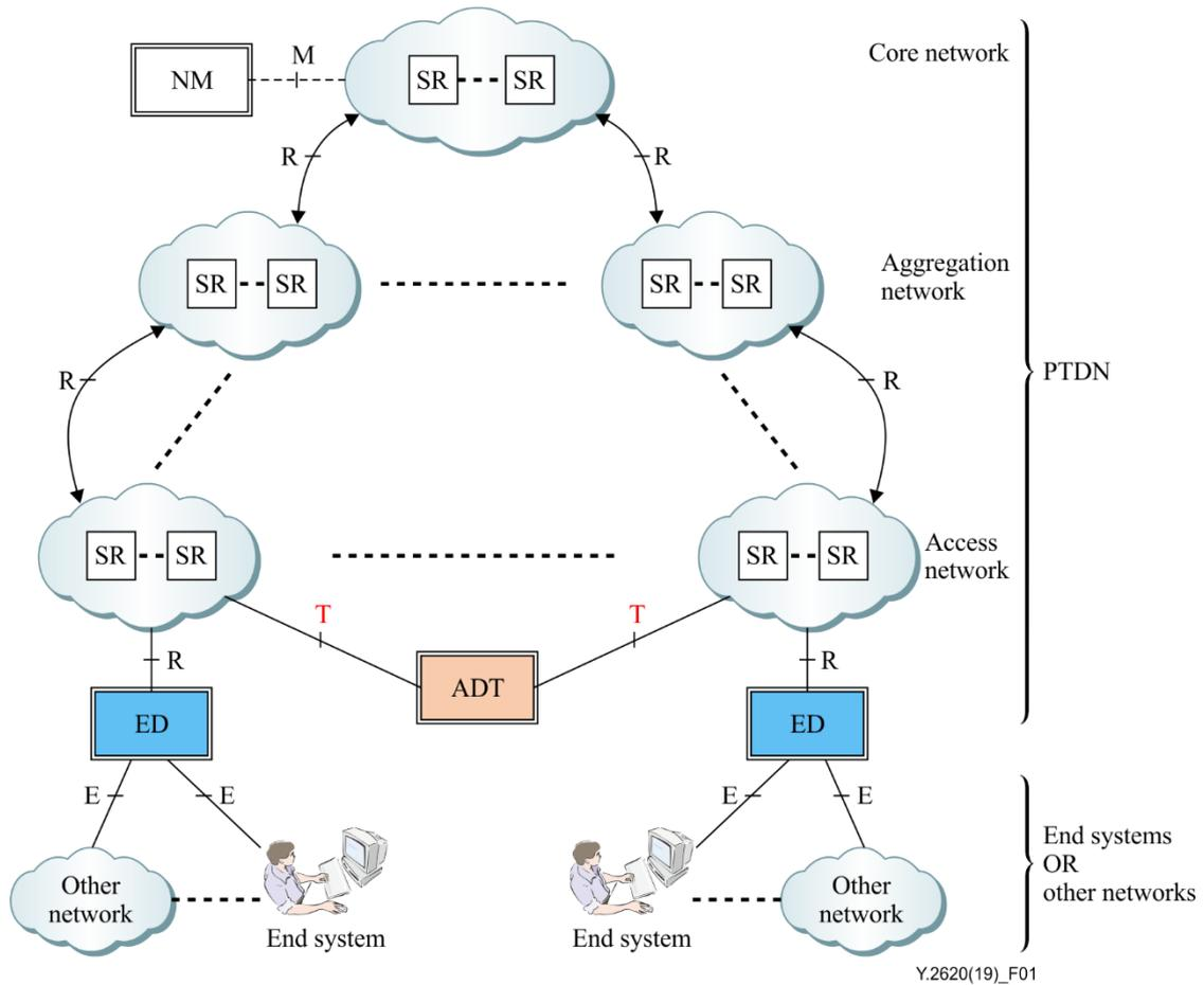
**Figure 1 – T interface in PTDN**
