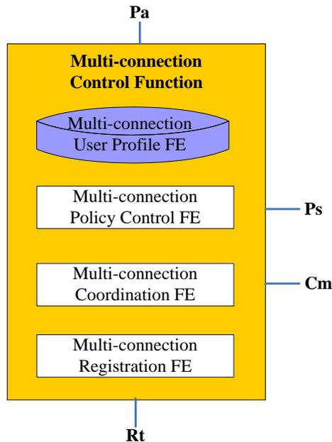
Figure 6-3 – Multi-connection control function
