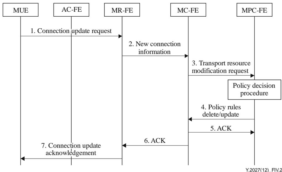
**Figure IV.2 – Deleting or updating a connection**
