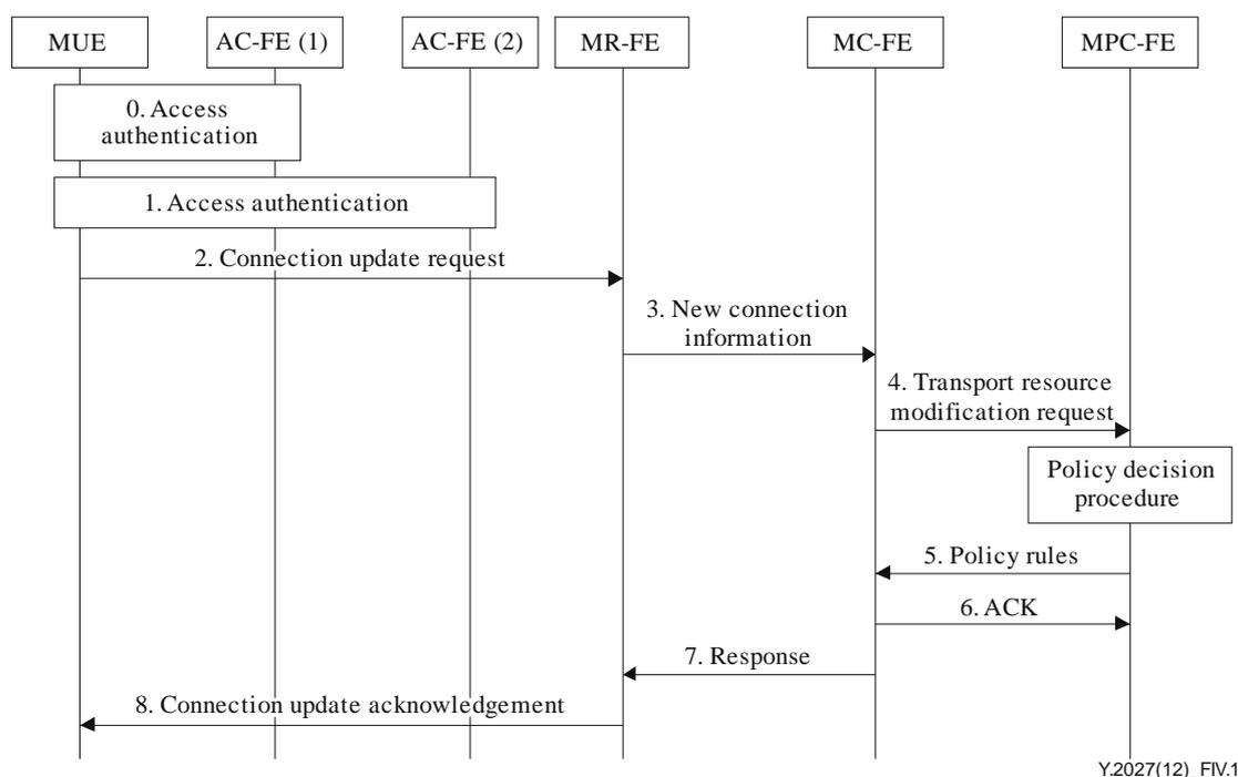
**Figure IV.1 – Adding a new connection**
