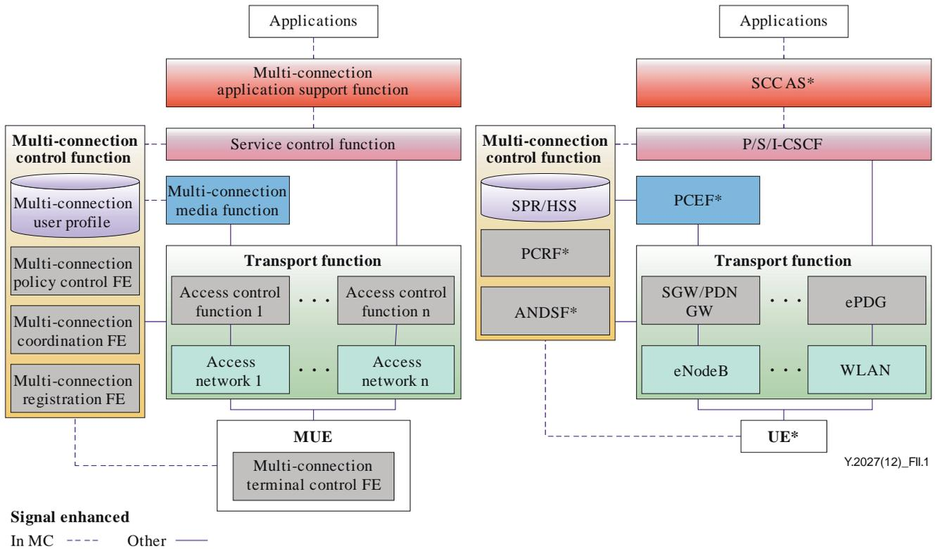
**Figure II.1 – Mapping of baseline to 3GPP EPC/IMS**
