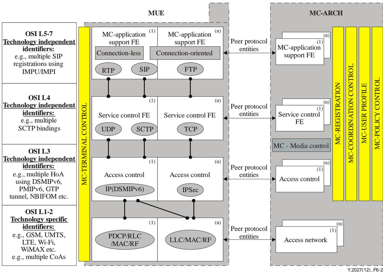
**Figure 6-2 – Functional entities supporting multi-connection architecture**
