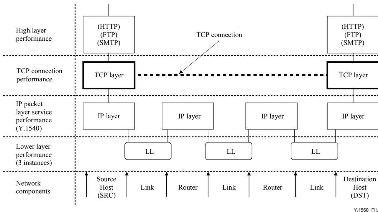
**Figure II.1/Y.1560 – Layered model of performance for TCP connection without a middlebox – example**
