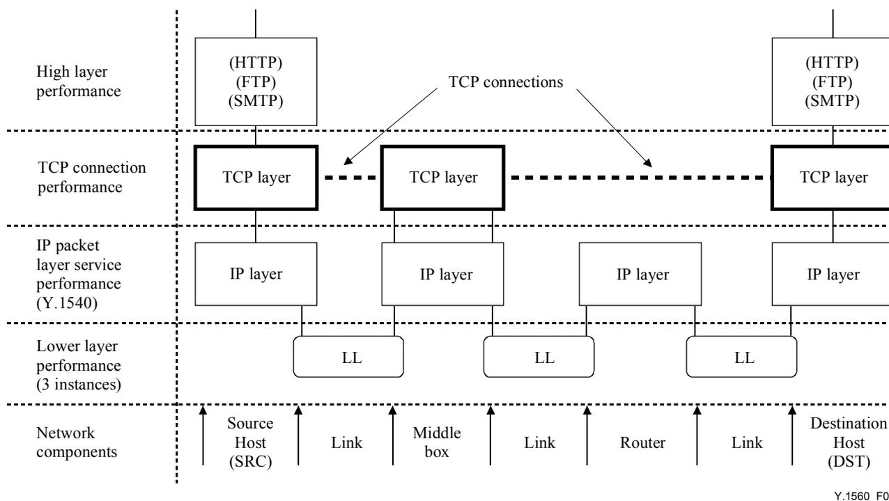
**Figure 1/Y.1560 – Layered model of performance for TCP connection with a middlebox – example**
