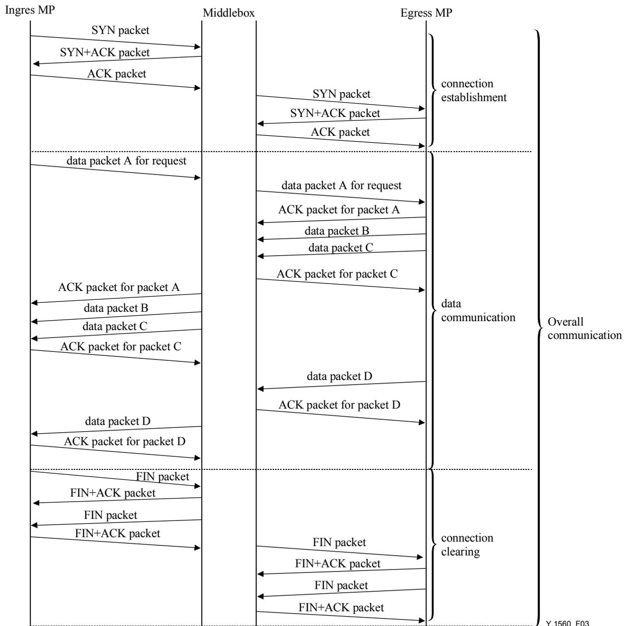
**Figure 3/Y.1560 – End-to-end timelines of TCP connections**
