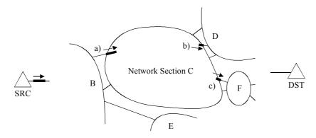
An IP packet from SRC to DST enters NS C, creates an ingress event, is fragmented, and creates two corresponding egress events, b) and c).
