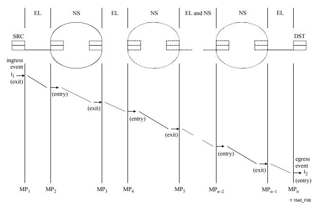
Figure 8/Y.1540 – IP packet transfer delay events (illustrated for the end-to-end transfer of a single IP packet)
