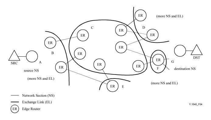
Figure 4/Y.1540 – IP network connectivity
