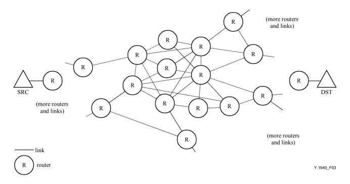
Figure 3/Y.1540 – IP network components
