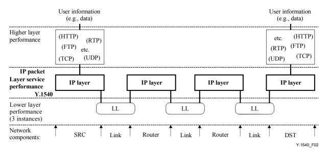
Figure 2/Y.1540 – Layered model of performance for IP service – Example
