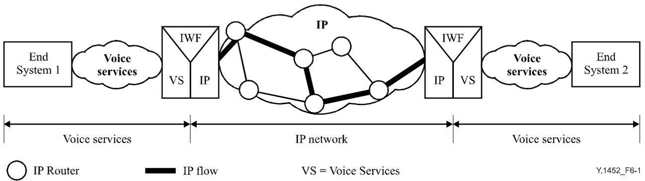
**Figure 6-1/Y.1452 – Reference architecture for voice trunking over IP**
