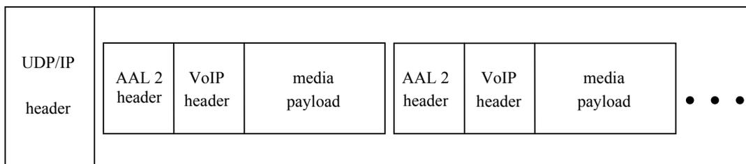
**Figure 11-1/Y.1452 – Encapsulation format for VoIP trunking**
