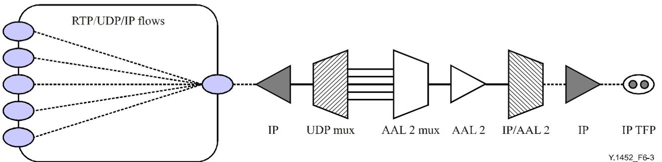
**Figure 6-3/Y.1452 – Functional architecture for multiplexing VoIP streams over IP networks**
