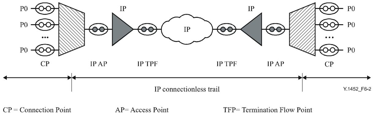
**Figure 6-2/Y.1452 – Functional architecture for multiplexing P0 channels over IP networks**
