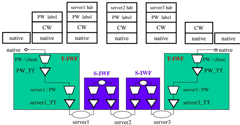
**Figure 6-5 – Encapsulations at different points of the functional diagram**
