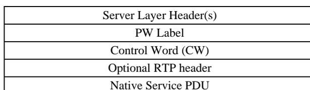
**Figure 8-4 – Server network PDU**
