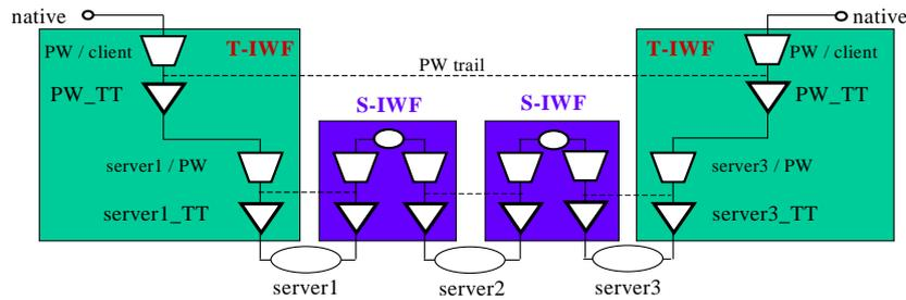
**Figure 6-2 – Functional diagram for multi-segment interworking for the multi-technology case**
