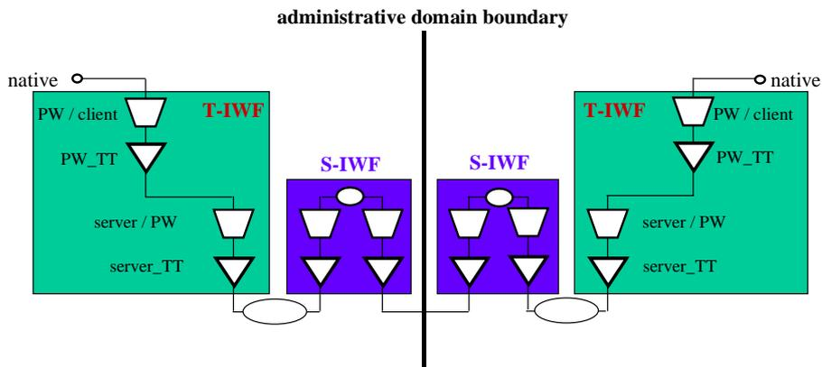
**Figure 6-3 – Functional diagram for multi-segment interworking for the multi-domain case**
