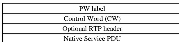
**Figure 8-1 – PW PDU**
