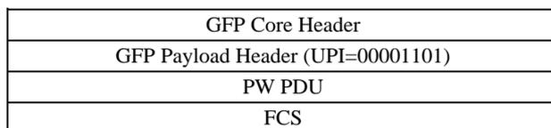
**Figure II.4 – Encapsulation format for PW over GFP**
