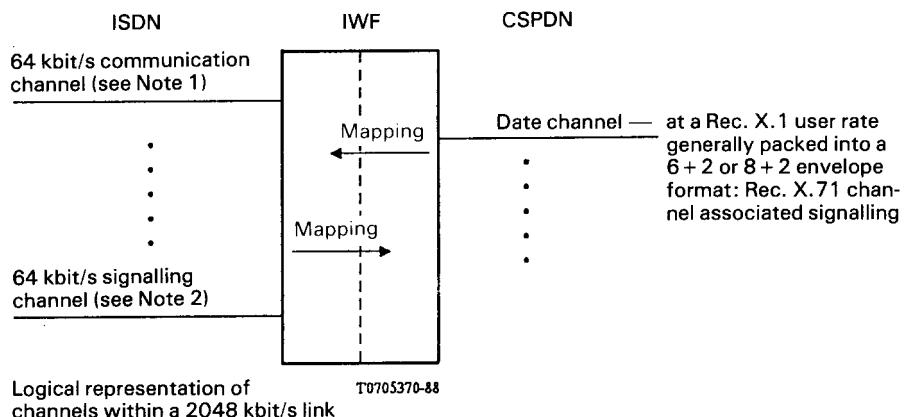
*Note 1* – 64 kbit/s communication channel bearing a data channel at a Rec. X.1 user rate (non-transparent ISDN connection).
