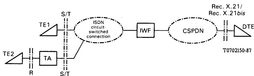
*Note – In cases where a TE1-type terminal is used, the bit stream at the S/T-interface complies with the Rec. X.30 frame structure.*
