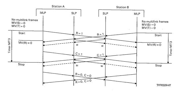
a) The SLP frame that acknowledges delivery of the multilink frame with R = 1.
