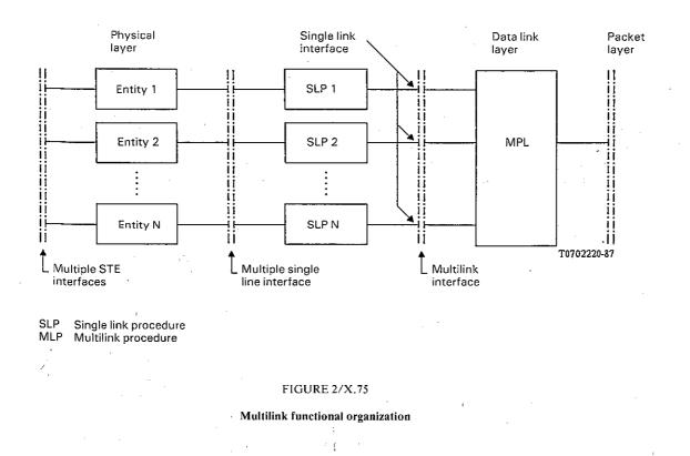
A multilink procedure (MLP) must perform the functions of distributing across the available SLPs, packets which are to be transmitted to the remote STE and of resequencing packets received from the remote STE for delivery to the packet layer.
