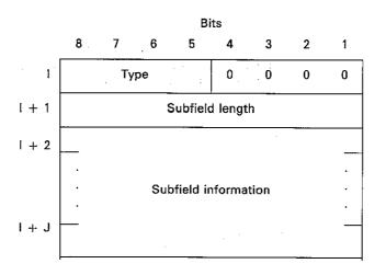
where I is the number of the initial octet of the subfield and (J - 1) is the number of octets of information in the subfield. The type semi–octet specifies the encoding format for the information of the subfield, as follows:
