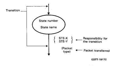
Note I – Each state is represented by an ellipse wherein the state name and number are indicated. Note 2 – Each state transition is represented by an arrow. The responsibility for the transition (STE-X or STE-Y) and the packet that has been transferred are indicated beside that arrow.
