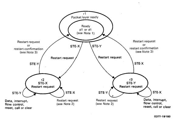
Note 1 - State p1 for virtual calls or state d1 for permanent virtual circuits.
