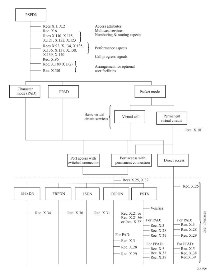
Figure 6/X.7 – X-series Recommendations discussing technical characteristics of packet switched data transmission services in PSPDNs
