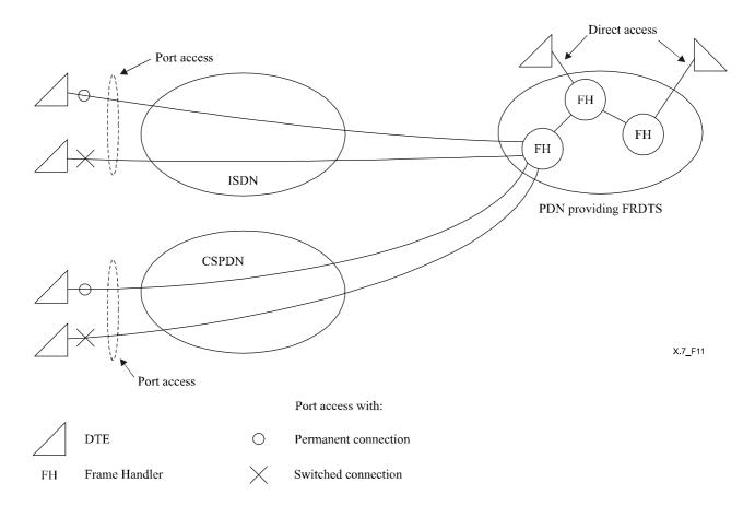
Figure 11/X.7 – Access mechanisms for frame relay data transmission services
