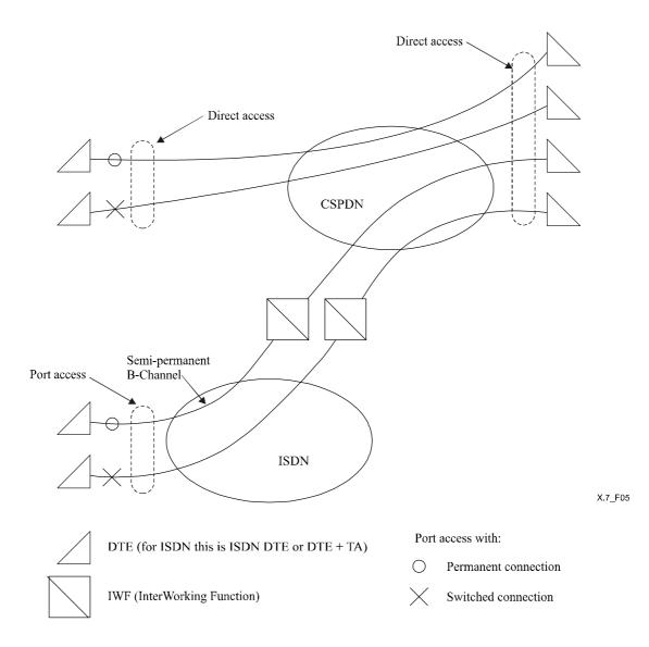
Figure 5/X.7 – Access mechanisms for circuit switched data transmission services provided by CSPDN
