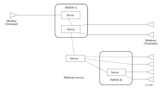
Figure 9/X.7 – Example of multicast server implementation
