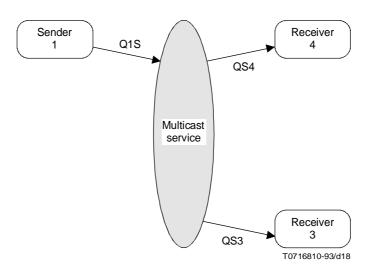
FIGURE 18/X.6 Model for data transfer – one-way communication
