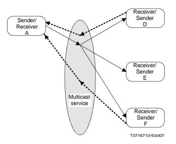
NOTE – Dashed lines indicate examples of return traffic from receiver/senders in the same multicast call.
