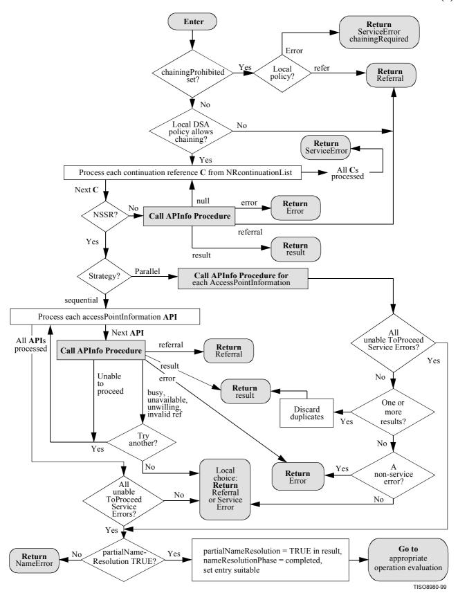
Figure 24 - Name Resolution Continuation Reference procedure
