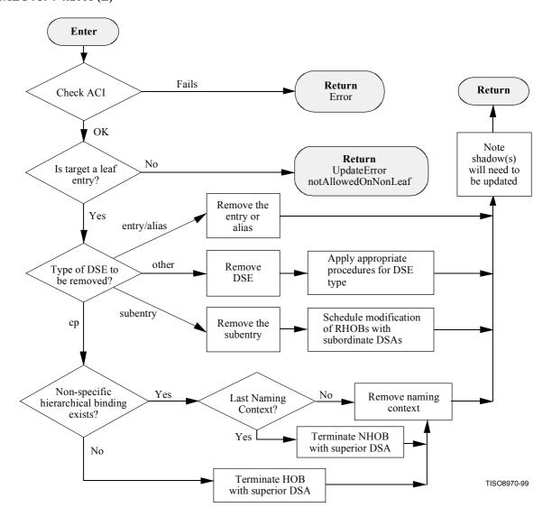
Figure 14 – Remove Entry procedure
