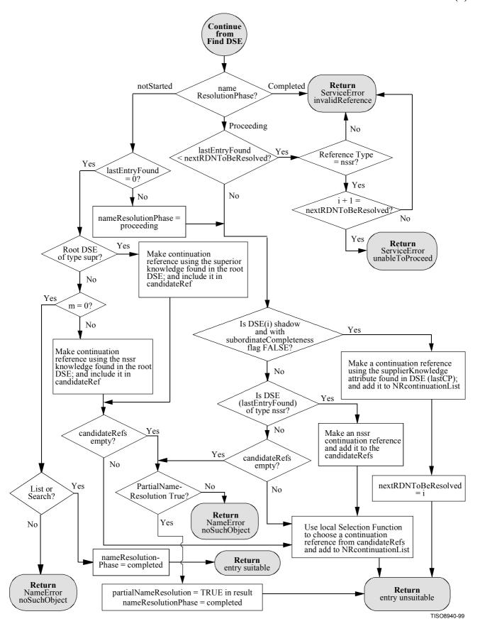
Figure 10 - Target Not Found sub-procedure
