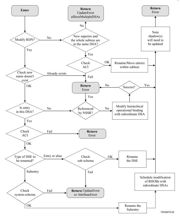
Figure 16 - Modify DN procedure
