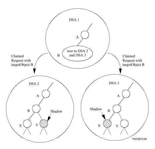
Figure 22 - Multi-chaining caused by NSSR during Name Resolution
