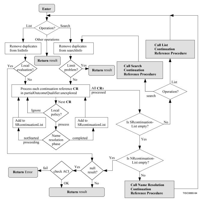
Figure 29 - Results Merging procedure
