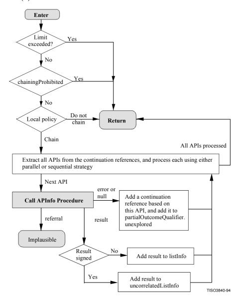
Figure 25 – List Continuation Reference procedure
