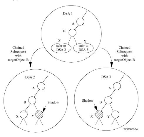
Figure 23 – Multi-chaining Request Decomposition using Subordinate References
