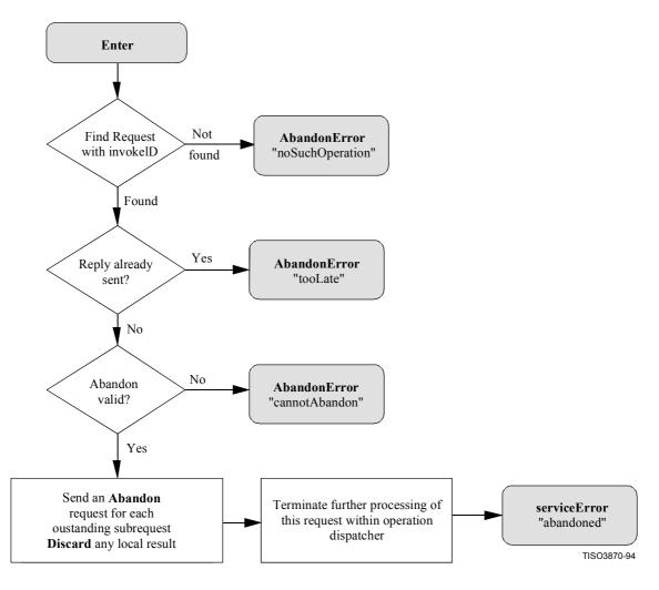
Figure 28 – Abandon procedure
