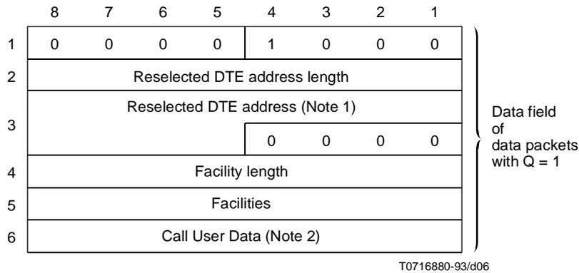
NOTE 1 – The figure is drawn assuming that the number of semi-octets in the DTE address is odd.
