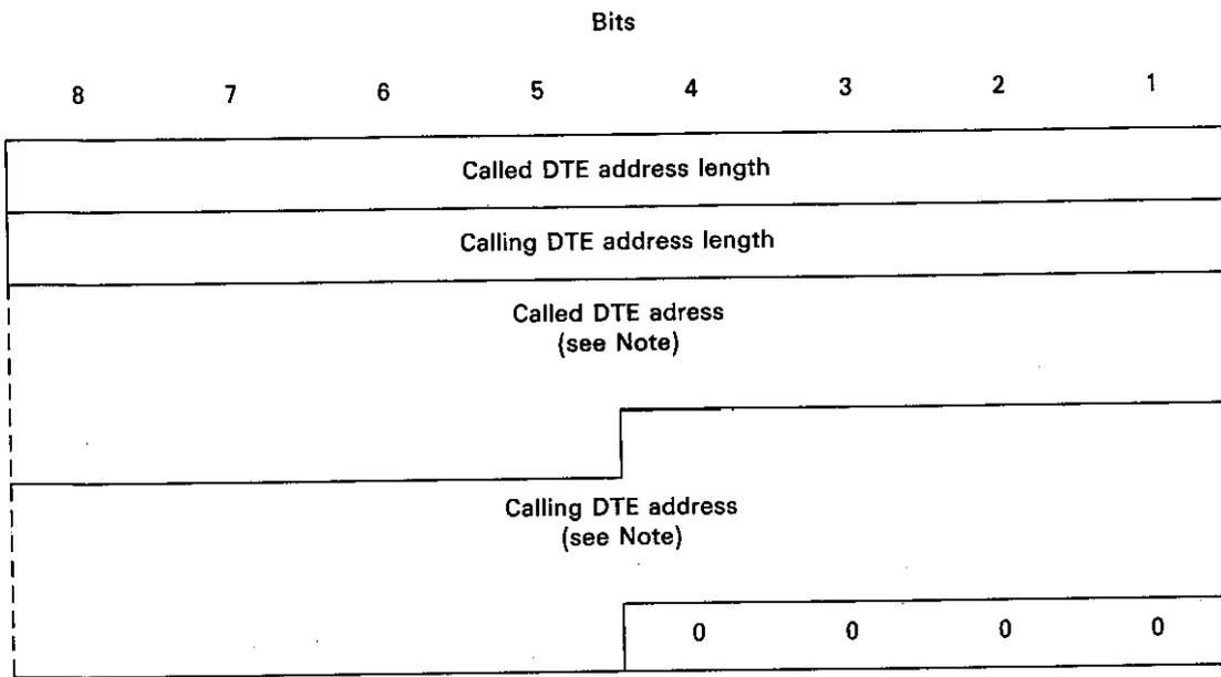
*Note* – The figure is drawn assuming the number of semi-octets present in the called DTE address field is odd and the number of semi-octets present in the calling DTE address field is even.
