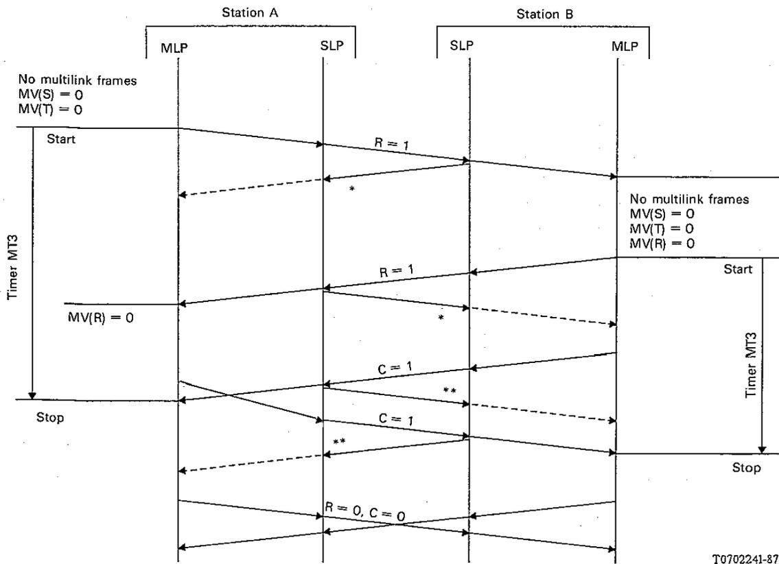
\* The SLP frame that acknowledges delivery of the multilink frame with  $R = 1$ .
