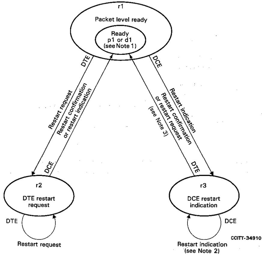
*Note 1* – State p1 for virtual calls or state d1 for permanent virtual circuits.
