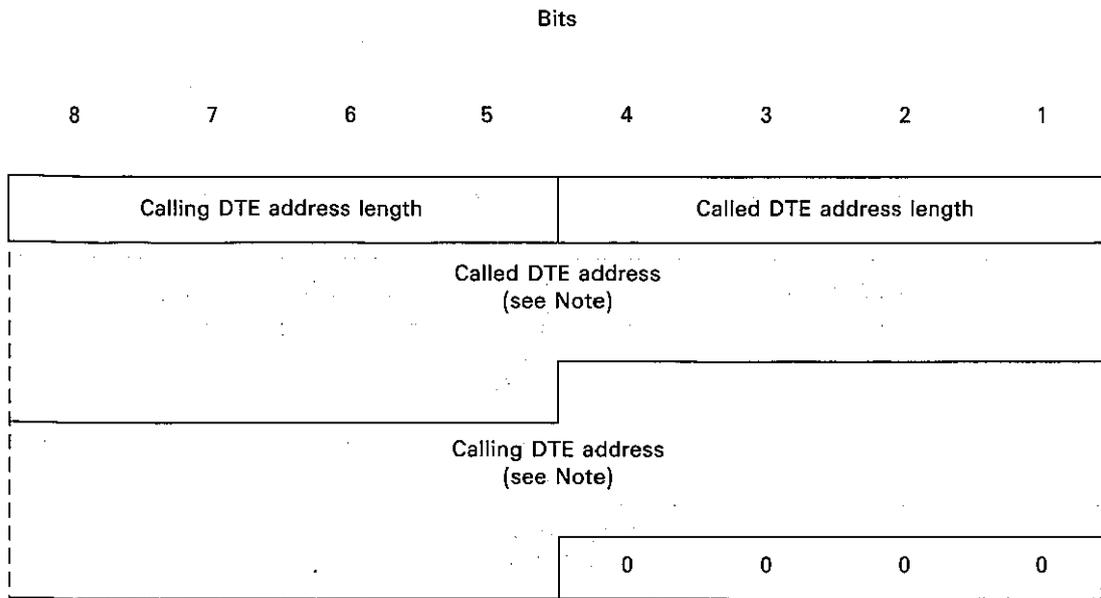
*Note* – The figure is drawn assuming the number of address digits present in the called DTE address field is odd and the number of address digits present in the calling DTE address field is even.
