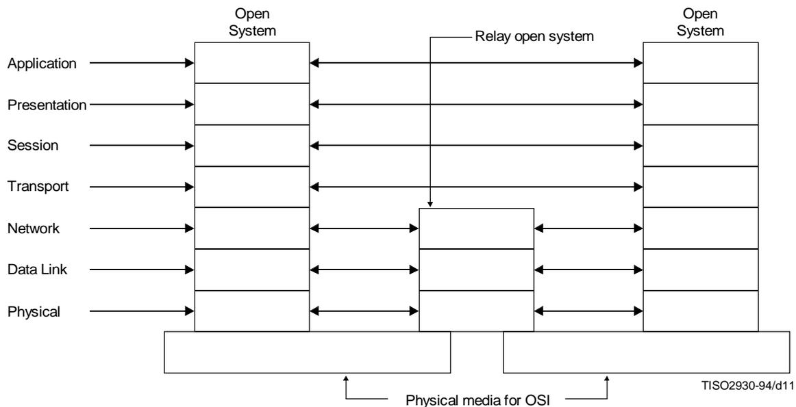
**Figure 12 – Communication involving relay open systems**
