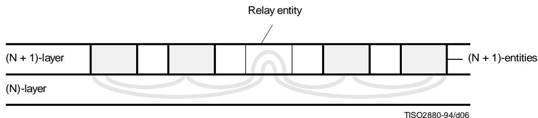
Figure 6 – Communication through a relay
