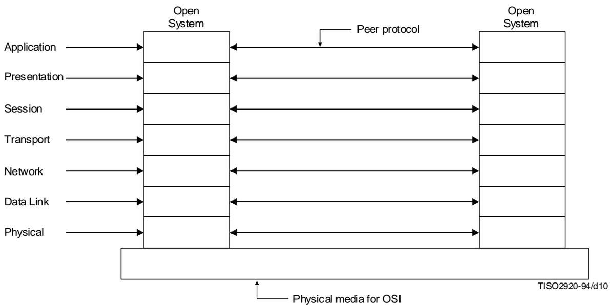
**Figure 11 – Seven layer reference model and peer protocols**
