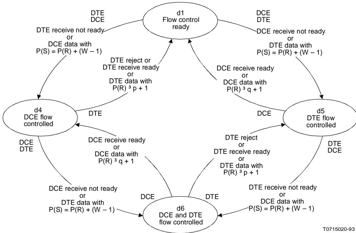
Note – Variables p and q represent the send sequence numbers of the last DTE data and DCE data packets transferred across the DTE/DCE interface, respectively.
