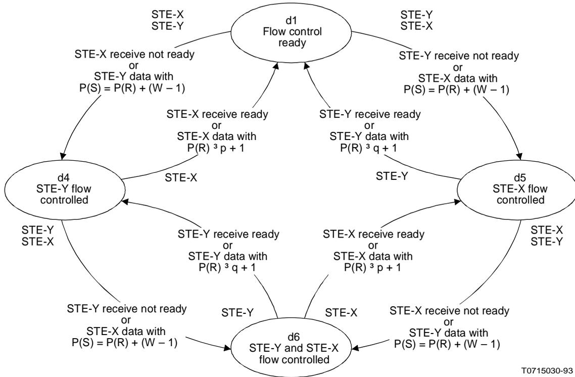
Note – Variables p and q represent the send sequence numbers of the last STE-X data and STE-Y data packets transferred across the STE-X/STE-Y interface, respectively.
