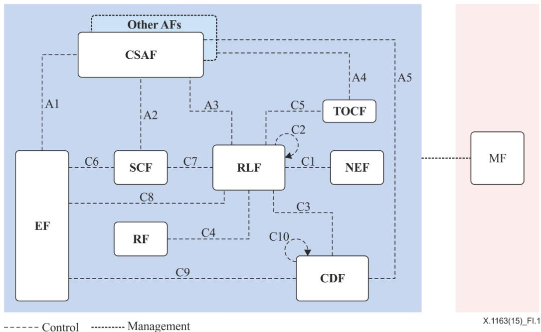
**Figure I.1 – DSN functional architecture**
