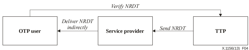
Figure 4 – Communication model for indirect NRDT
