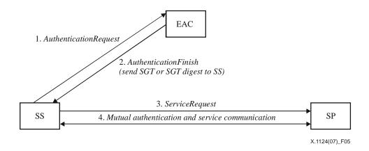
Figure 5 – Authentication inquiring and derived key transportation mechanism based on Kerberos
