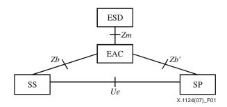
Figure 1 – Authentication model in mobile end-to-end data communication
