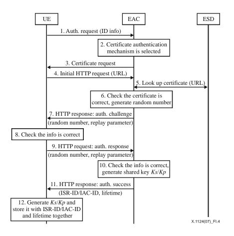
Figure I.4 – Authentication mechanism based on certificate use
