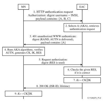
Figure I.2 – HTTP digest AKA used in 3GPP2
