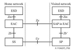
Figure 2 – Authentication model for accessing service in visited network
