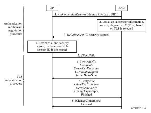
Figure I.3 – TLS based on certificate authentication mechanism use
