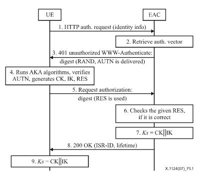
Figure I.1 – HTTP digest AKA used in 3GPP
