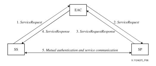
Figure 6 – Authentication inquiring and derived key agreement mechanism based on Mediation
