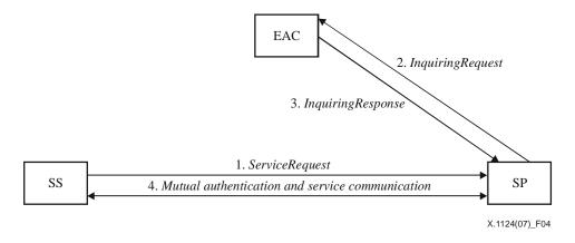
Figure 4 – Authentication enquiring and derived key generation mechanism based on GBA
