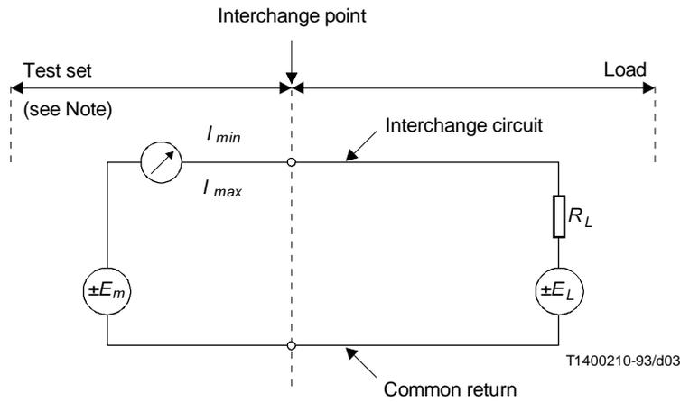
NOTE – The internal resistance of the ammeter shall be much less than the load resistance ( $R_L$ ).
