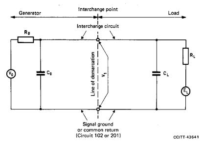
$V_0$  is the open-circuit generator voltage.
