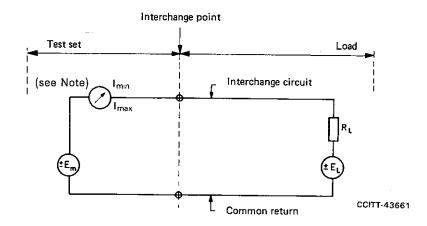
Note – The internal resistance of the ammeter shall be much less than the load resistance  $(R_L)$ .
