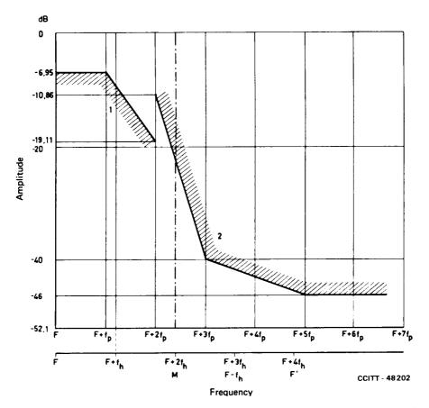
F = carrier frequency of a channel $f_p = \text{frequency of modulation} = 100 \text{ Hz}$  M = centre line between adjacent channels
