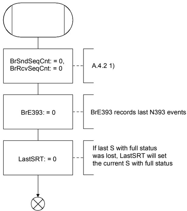
Figure A.13/Q.933 – Procedure InitResponse
