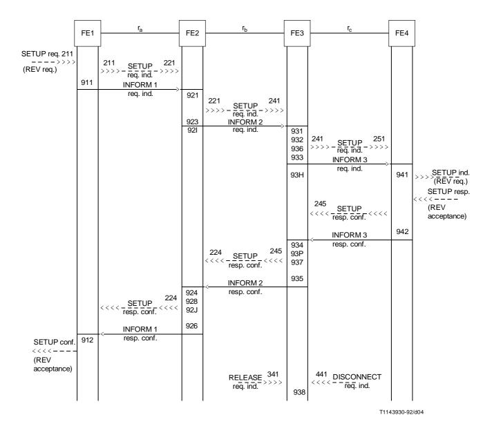
FIGURE 3-4/Q.86 Successful information flows for Case A (Transfer mode)
