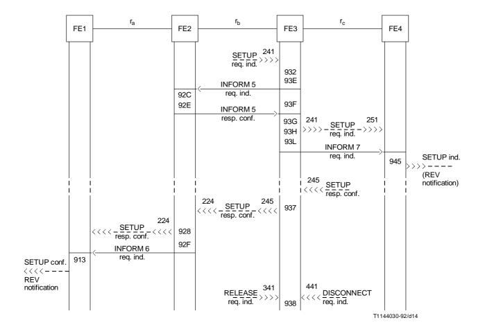
FIGURE 3-14/Q.86 Successful information flows for Case D (Transfer mode)
