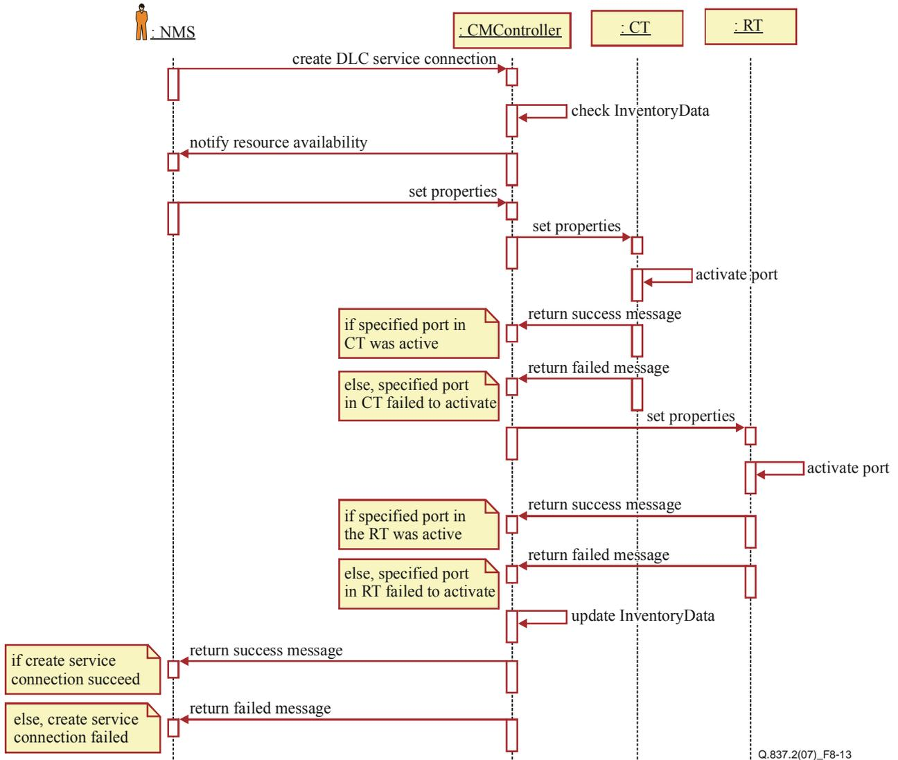
Figure 8-13 – Create DLC service connection sequence diagram
