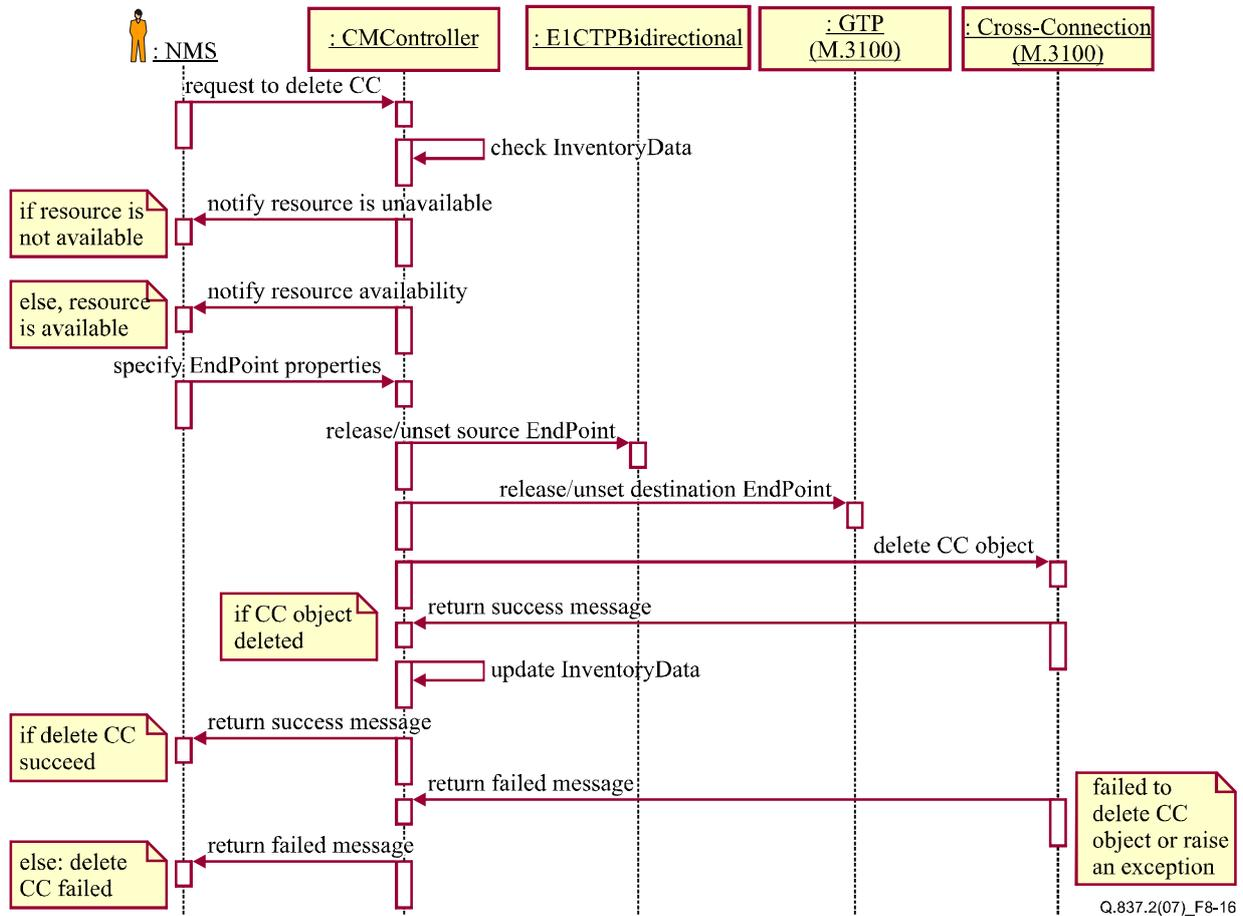
Figure 8-16 – Remove SDH cross-connection sequence diagram
