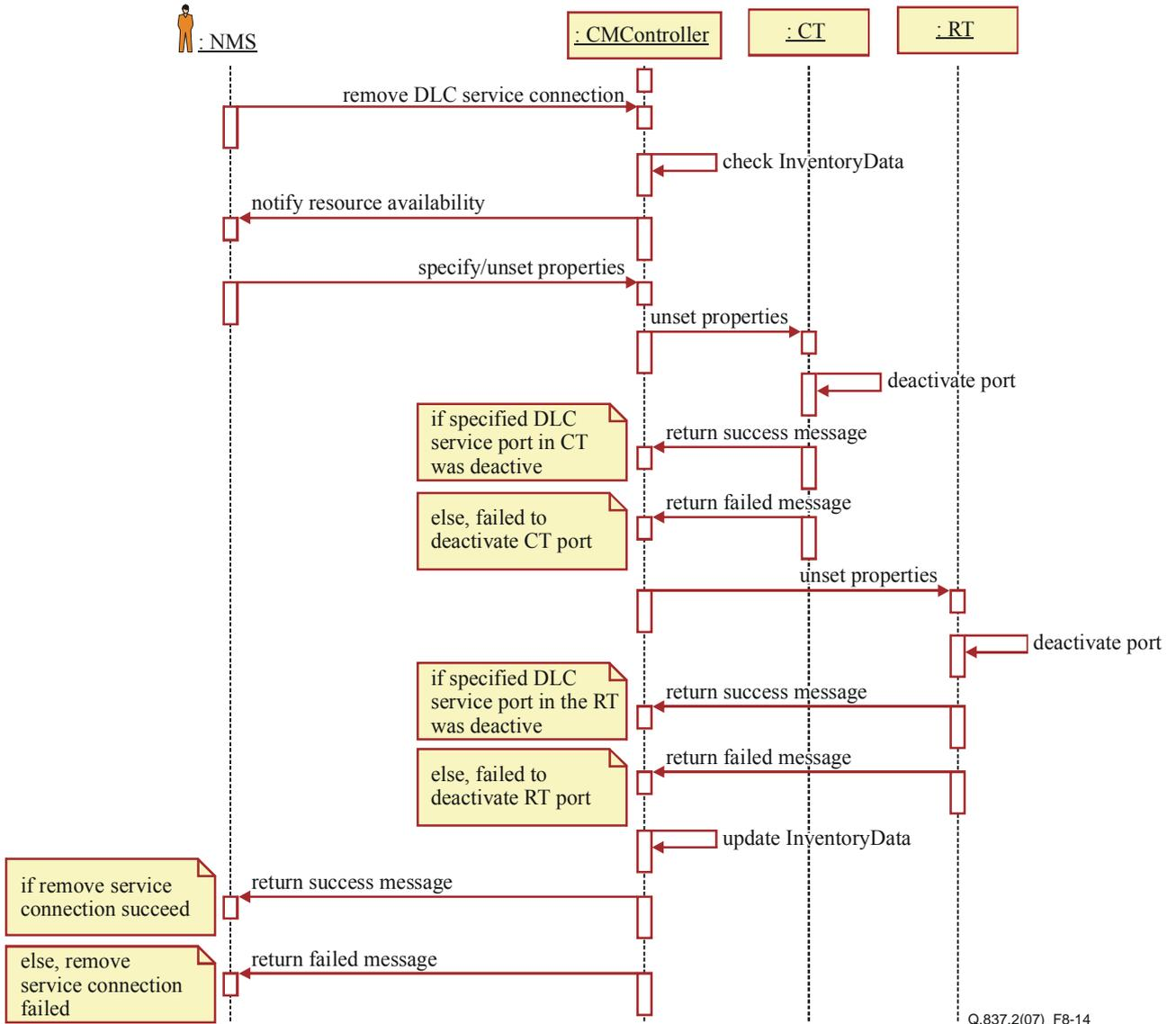
Figure 8-14 – Remove DLC service connection sequence diagram
