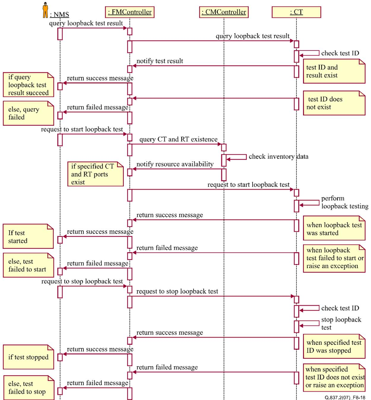
Figure 8-18 – DLC loopback test sequence diagram
