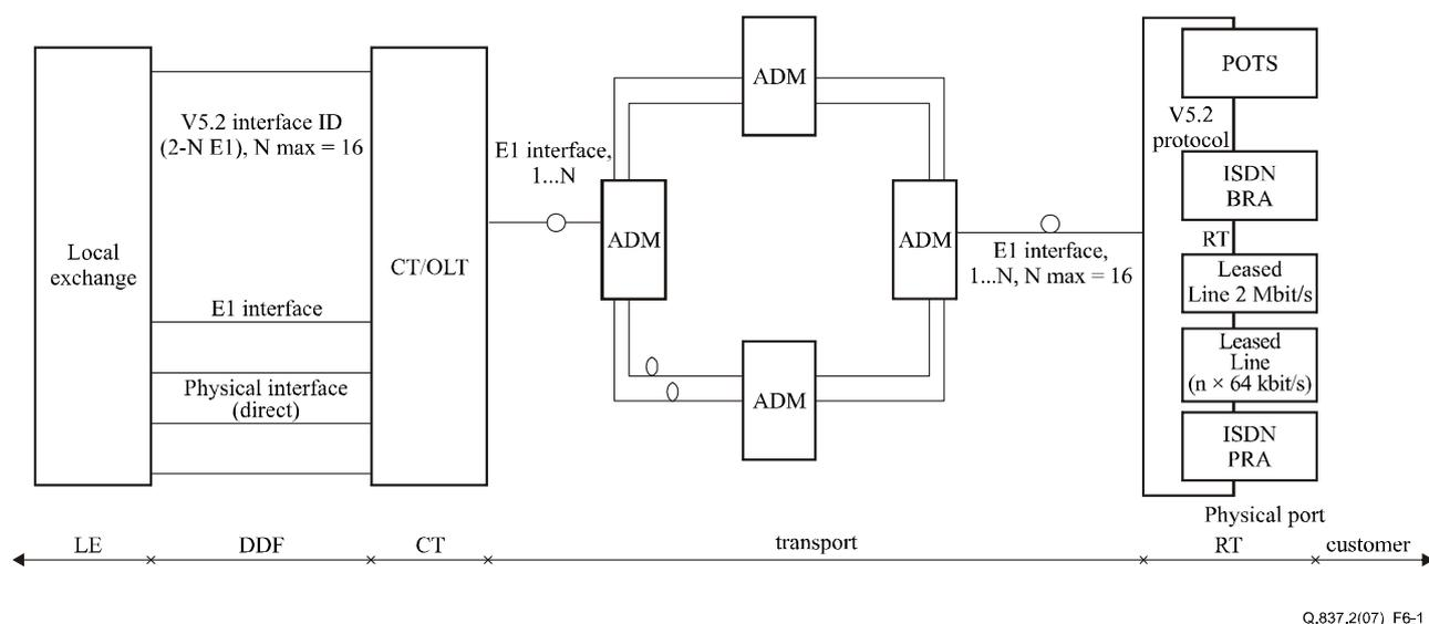
**Figure 6-1 – The general configuration of DLC and SDH system**
