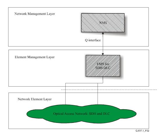
Figure 2/Q.837.1 – SDH and DLC management layers
