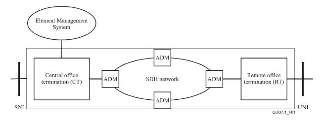
Figure 1/Q.837.1 – SDH and DLC network elements
