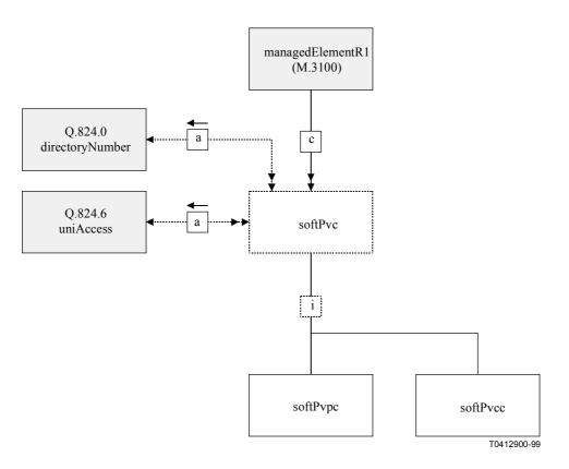
Figure 3/Q.824.7 – Entity relationship diagram – soft PVCs
