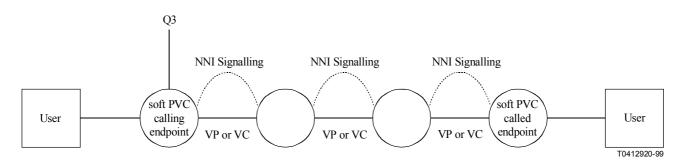
Figure A.1/Q.824.7 – Soft PVC Configuration
