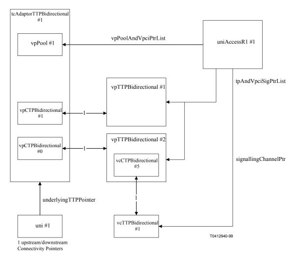
NOTE 1 – The use of #0 for the signalling VP and #5 for the signalling VC is deliberate so that the RDNs match the signalling VPI and VCI.
