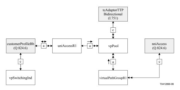
Figure 2/Q.824.7 – Entity relationship diagram – switched virtual paths
