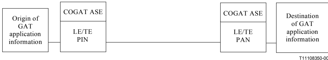
Figure 2/Q.765.4 – One example of a bearer unrelated communication between two nodes for a GAT application and its relationship with the public NNI's PIN/PAN concept
