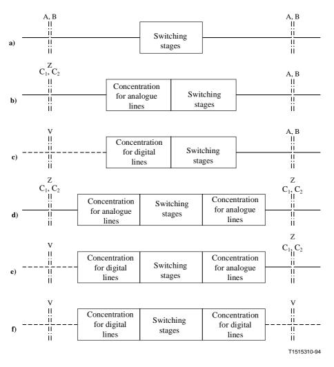
Figure 3/Q.551 – Exchange configurations as used for estimation of round trip absolute group delay
