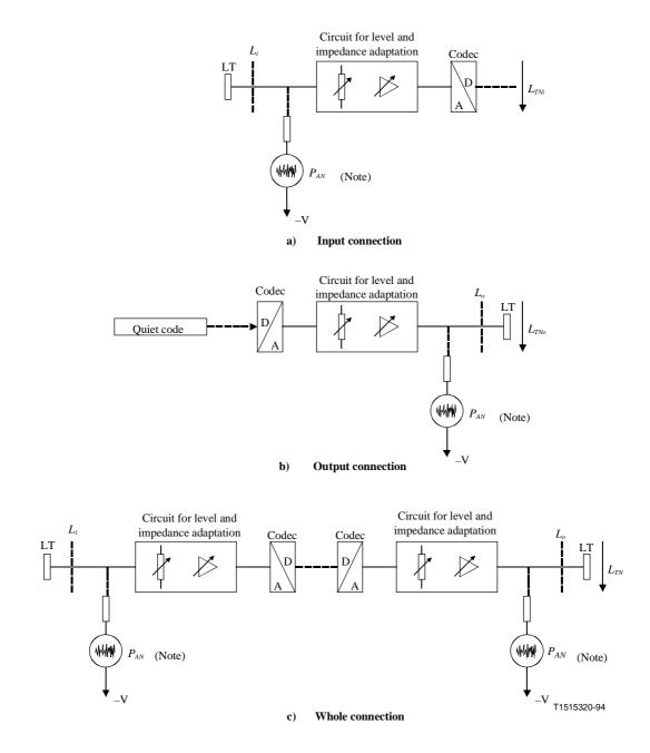
NOTE  $-P_{AN}$  to be considered for Z-interface with feeding and C-interfaces with signalling on the speech wires. LT = Line termination with matched conditions. All other abbreviations are in line with the text of this Recommendation.
