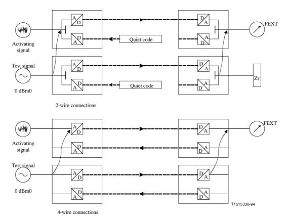
Figure 5/Q.551 – Measurement of crosstalk between two connections
