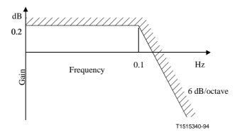
Figure 6/Q.551 – Exchange transfer function mask
