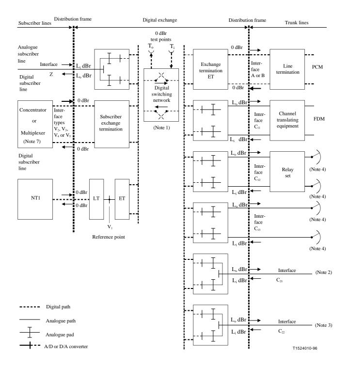
NOTE 1 - Digital loss pads, if required, may be located in the switching network or the exchange terminals (see 1.2.4.1).
