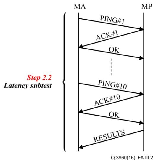
Figure III.2 – Example of latency test
