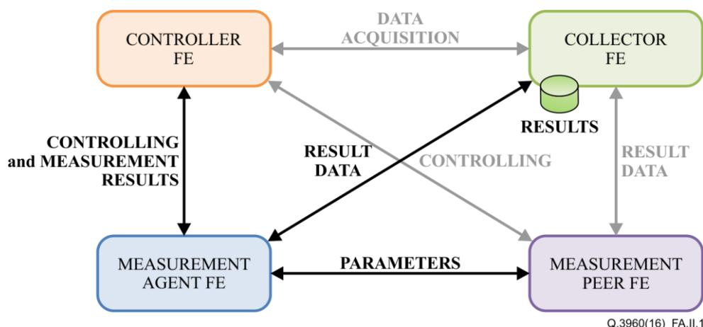
**Figure II.1 – The functional architecture of the basic measurement system**
