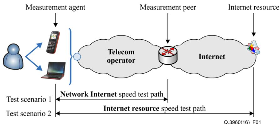
**Figure 1 – Global scenario and test definition**
