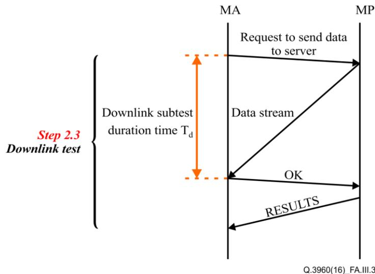
**Figure III.3 – Example of downlink test**
