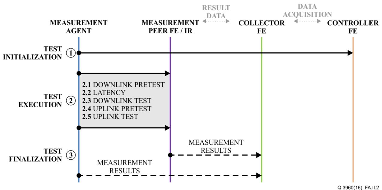
**Figure II.2 – The workflow of the measurement system**
