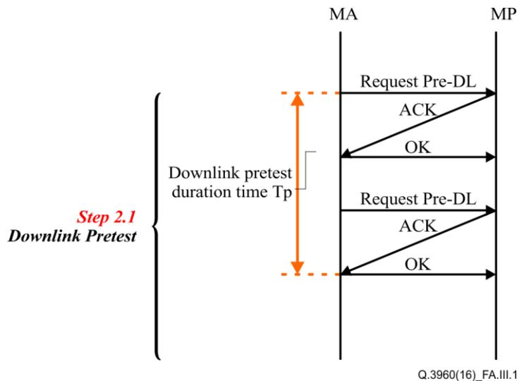
Figure III.1 – Example of downlink pre-test
