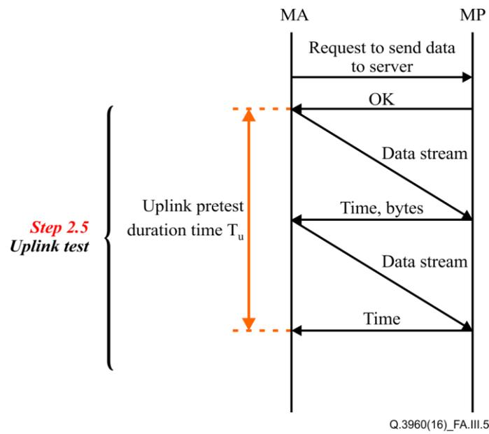
**Figure III.5 – Example of uplink test**
