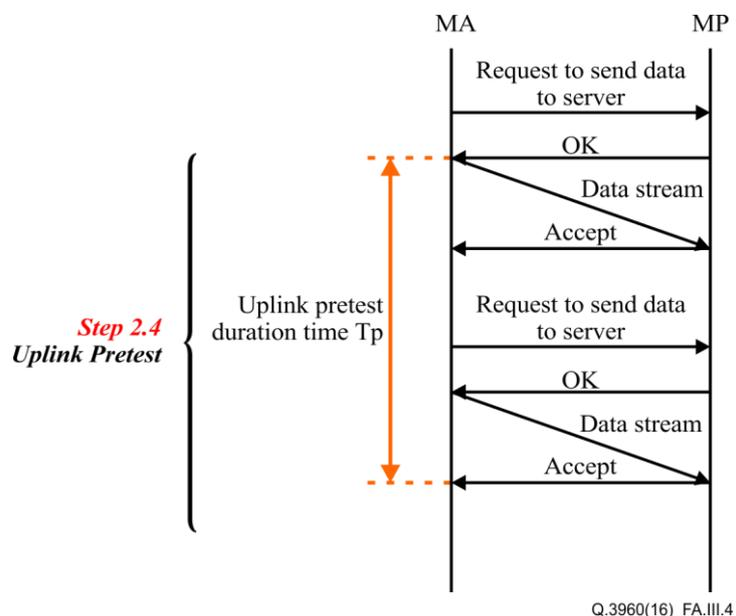
**Figure III.4 – Example of uplink pre-test**
