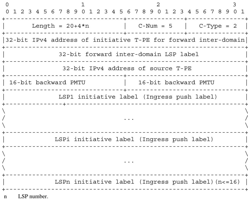
**Figure 8-13 – IPv4 backward LSP connection information object content**
