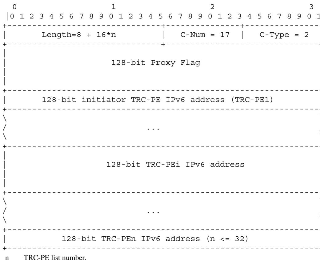
**Figure 8-31 – IPv6 TRC-PE sequence object content**
