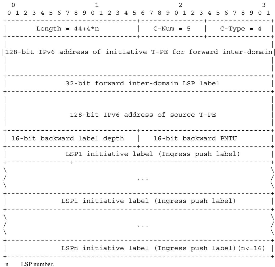
**Figure 8-15 – IPv6 backward LSP connection information object content**
