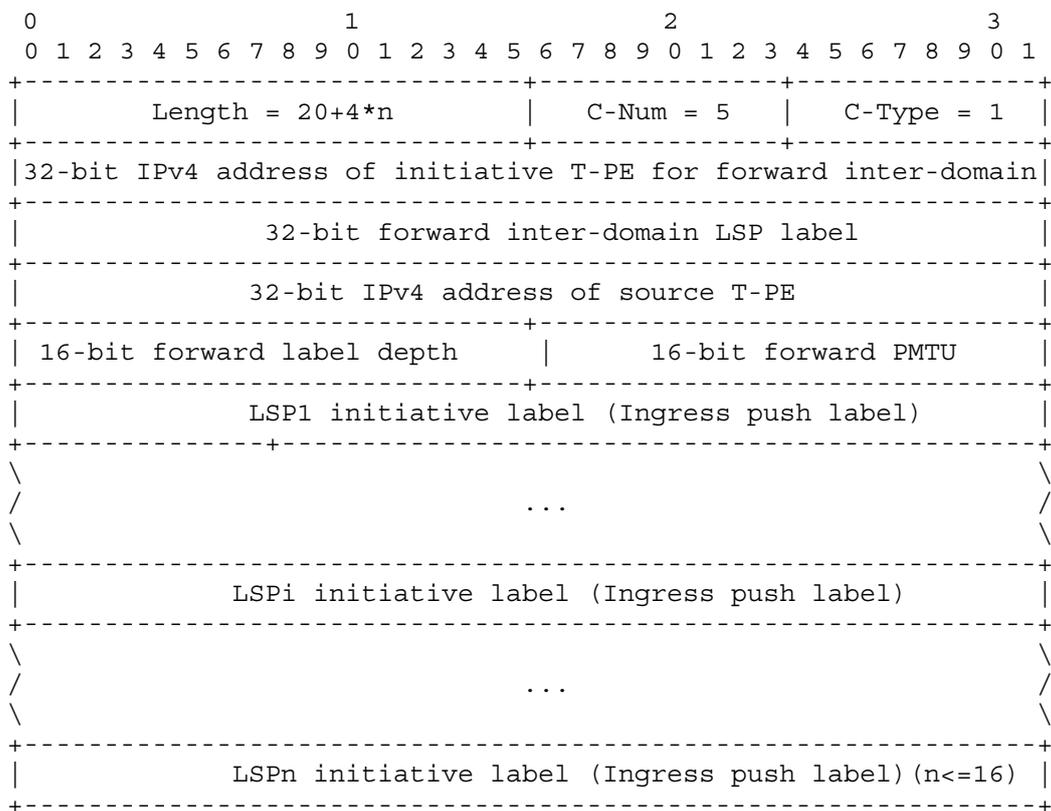
**Figure 8-12 – IPv4 forward LSP connection information object content**
