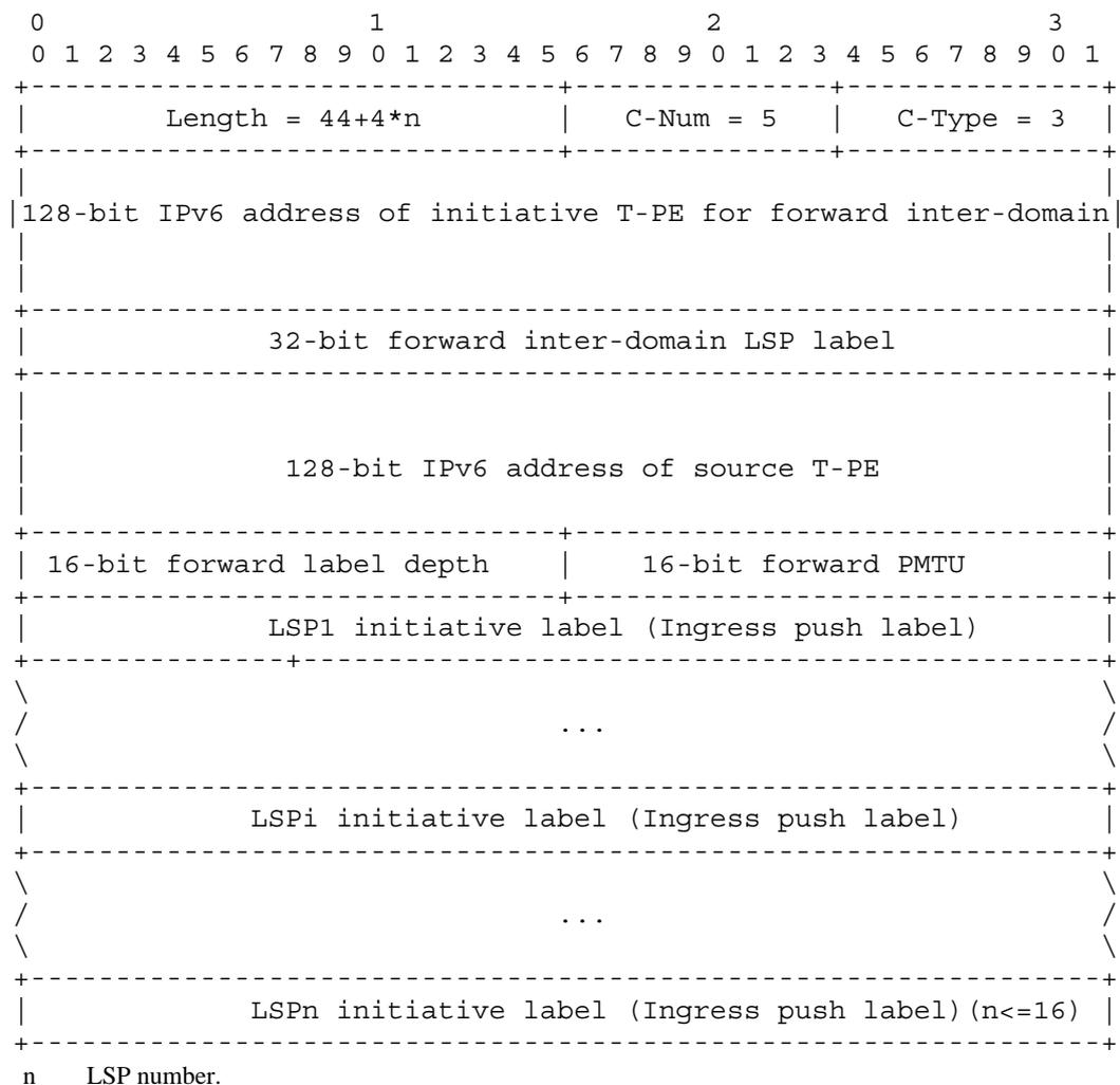
**Figure 8-14 – IPv6 forward LSP connection information object content**
