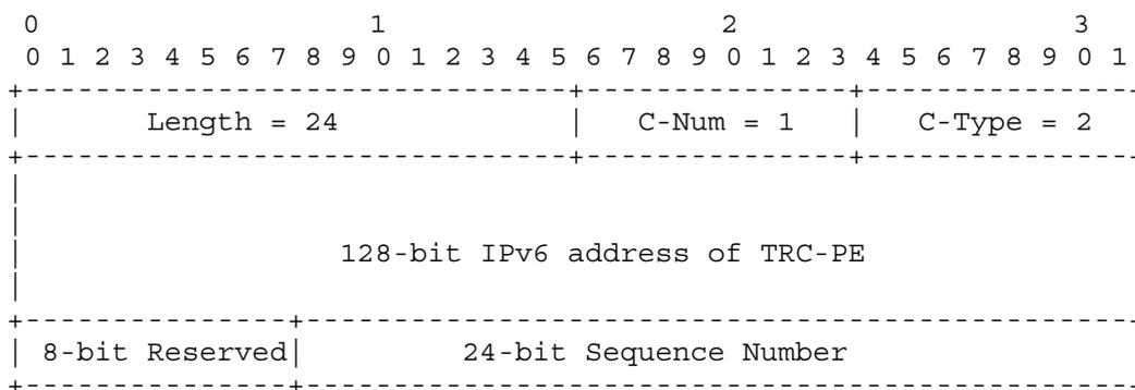
Figure 8-6 – IPv6 connection id object content
