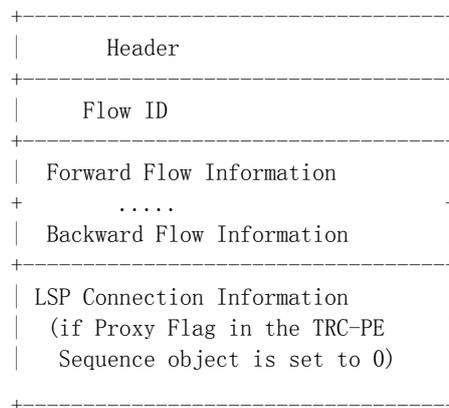
**Figure 8-23 – Flow profile for MPLS case object content**
