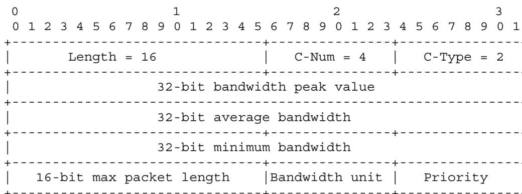
Figure 8-11 – Backward flow traffic descriptor object content
