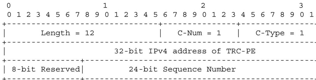
Figure 8-5 – IPv4 connection id object content
