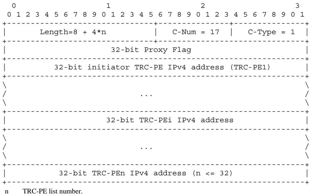
**Figure 8-30 – IPv4 TRC-PE sequence object content**
