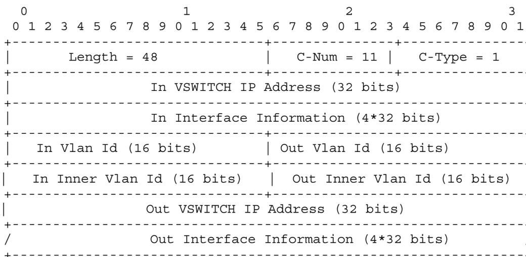
**Figure 8-21 – V-switching connection information object content**
