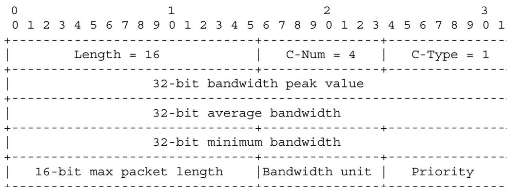
Figure 8-10 – Forward flow traffic descriptor object content
