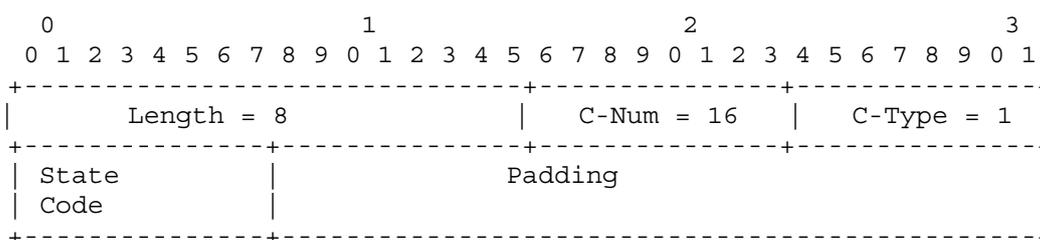
Figure 8-26 – Connection resource state object content
