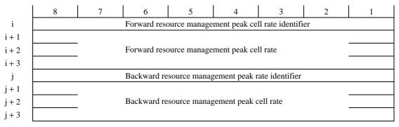
Figure 1/Q.2723.4 – Extended coding of the Additional ATM cell rate parameter
