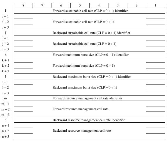
Figure 2/Q.2723.4 – Extended coding of the Minimum ATM cell rate parameter
