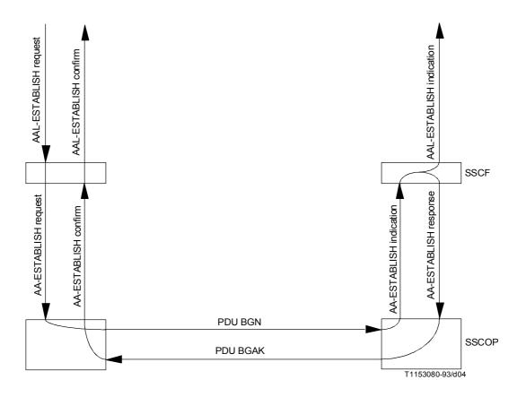
FIGURE 1.1/Q.2130 Sequences for establishment of AAL connection
