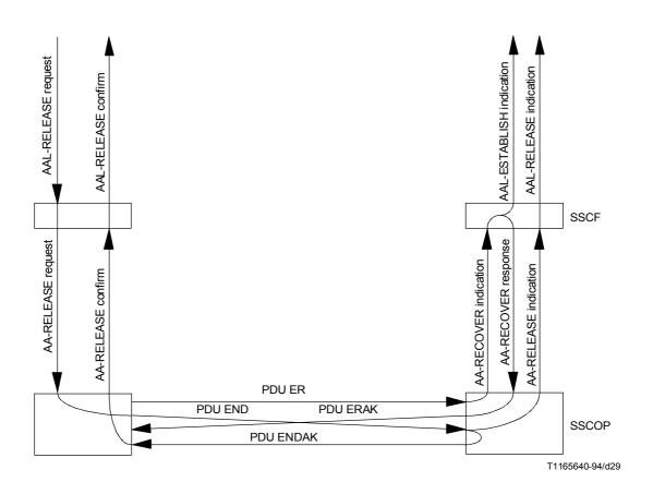
FIGURE 1.26/Q.2130 Sequences for recovery of AAL connection followed by connection release
