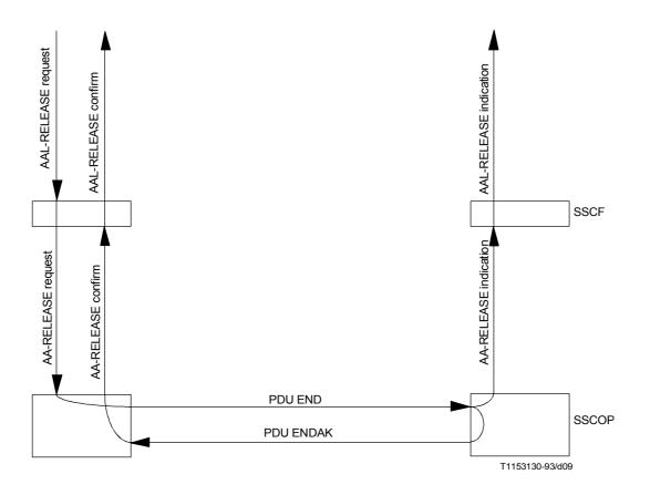
FIGURE 1.6/Q.2130 Sequences for release of AAL connection
