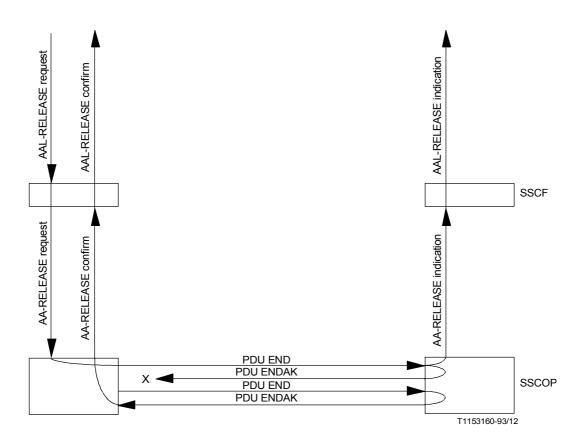
FIGURE 1.9/Q.2130 Sequences for release of AAL connection in case of corruption of PDU ENDAK
