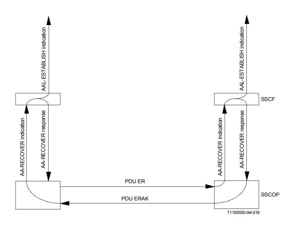
FIGURE 1.15/Q.2130 Sequences for recovery of AAL connection
