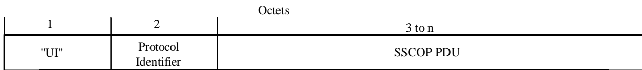
Figure 2/Q.2119 – PDU format to embed an SSCOP PDU in a frame relay SDU
