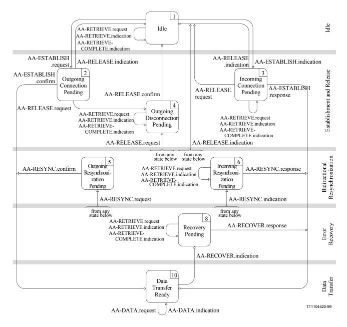
NOTE – The SSCOPMCE connection state Recovery Pending (State 8) covers the SSCOPMCE states Recovery Response Pending (State 8) and Incoming Recovery Pending (State 9). Which of these states applies is not visible at the boundary between SSCOPMCE and its user. The State Outgoing Recovery Pending (State 7) is never visible at the boundary between SSCOPMCE and its user.
