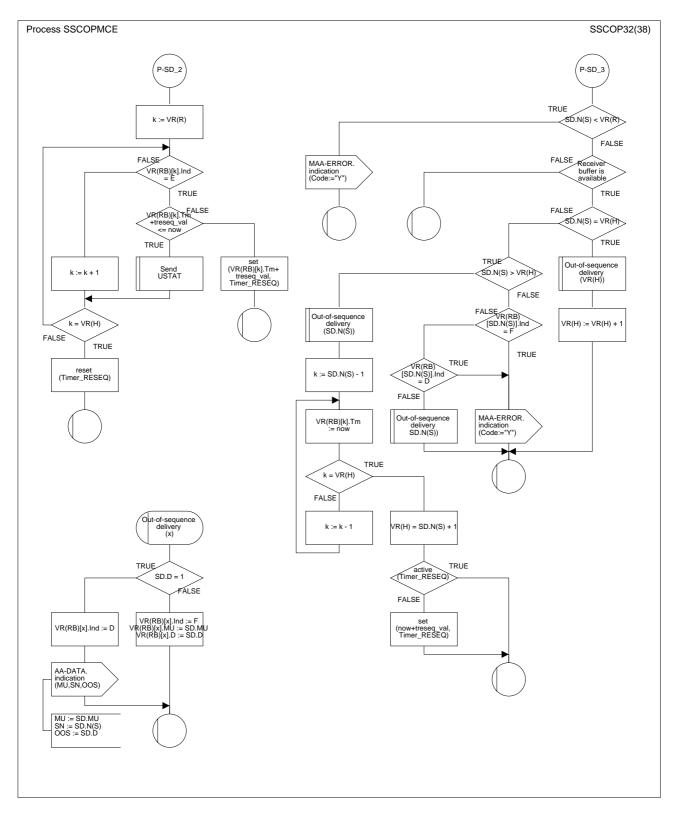
Figure 22/Q.2111 – SDL diagram of the multilink SSCOPMCE protocol entity (sheet 32 of 38)
