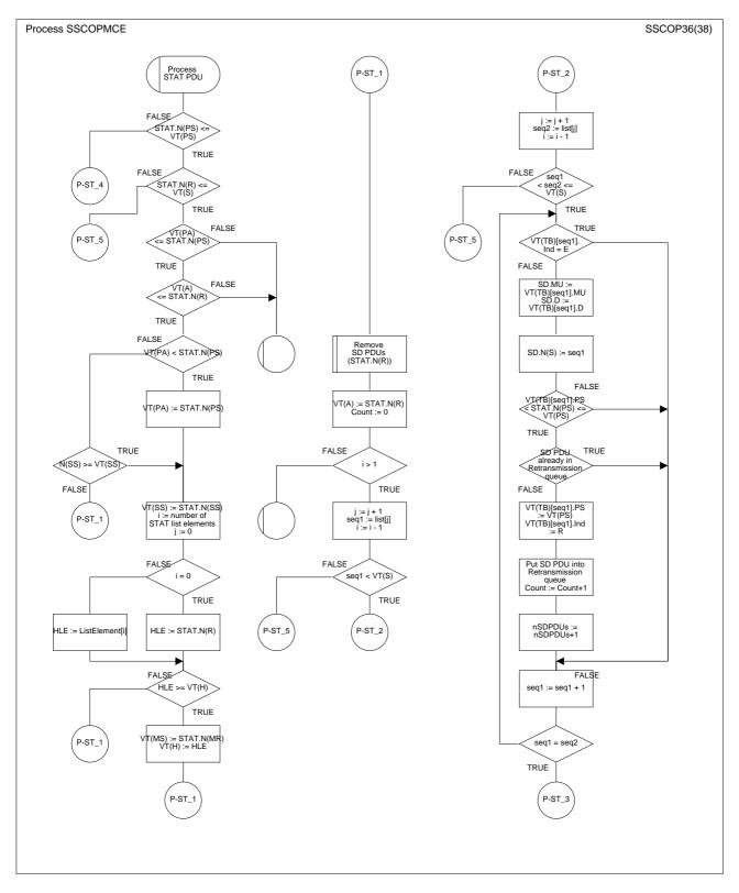
Figure 22/Q.2111 – SDL diagram of the multilink SSCOPMCE protocol entity (sheet 36 of 38)
