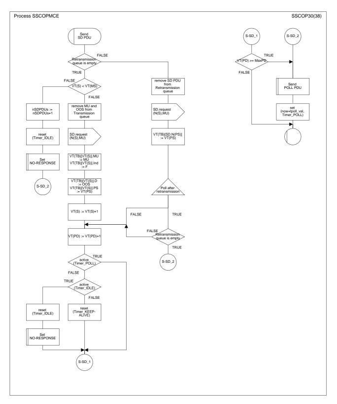
Figure 22/Q.2111 – SDL diagram of the multilink SSCOPMCE protocol entity (sheet 30 of 38)
