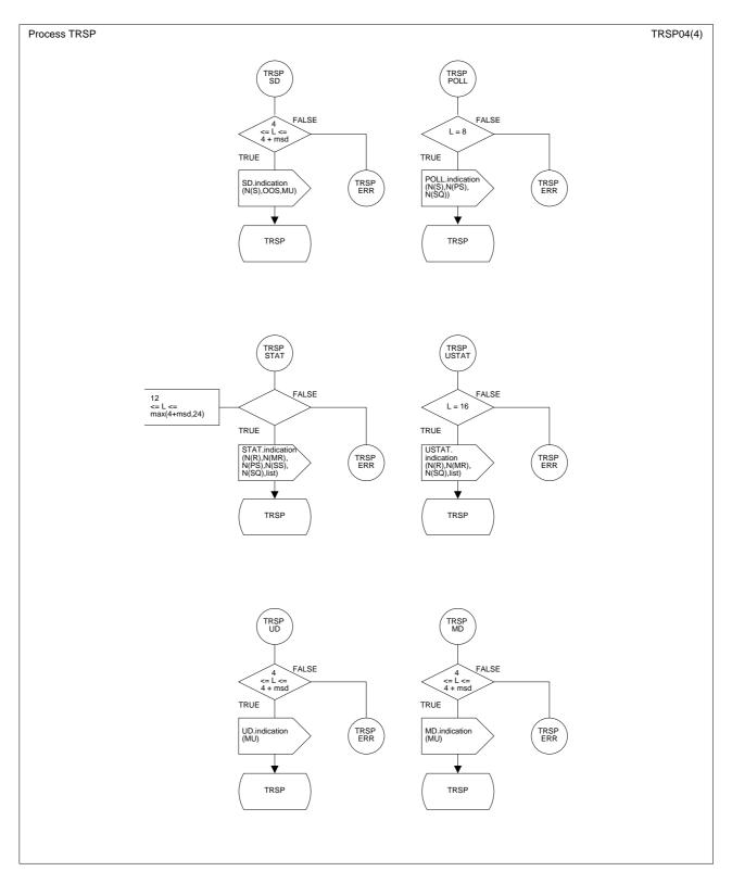
Figure B.1/Q.2111 – SDL diagram of the ancillary process TRSP (sheet 4 of 4)
