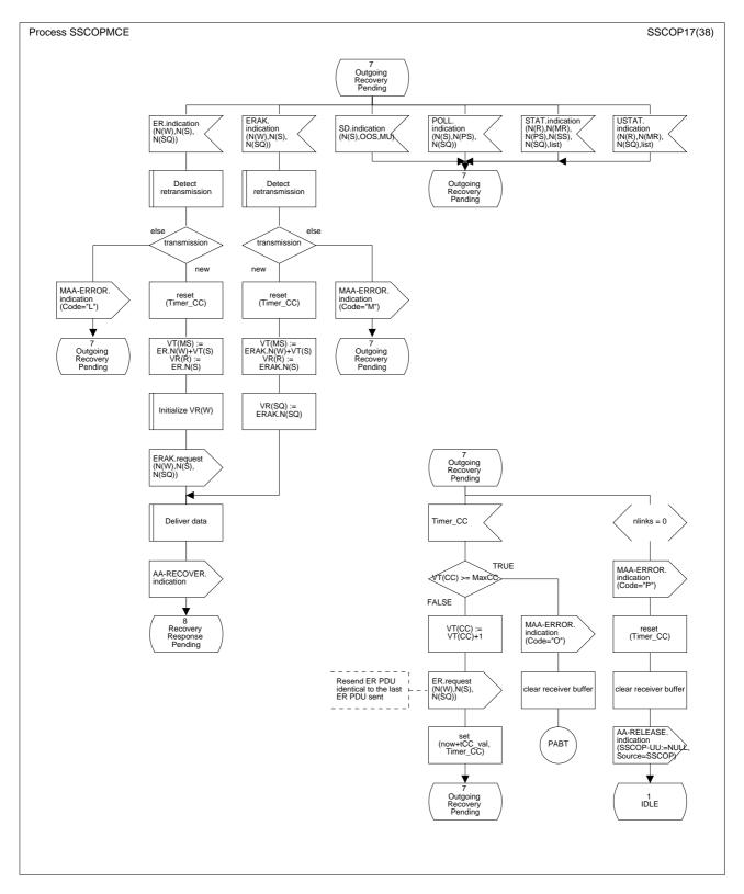
Figure 22/Q.2111 – SDL diagram of the multilink SSCOPMCE protocol entity (sheet 17 of 38)
