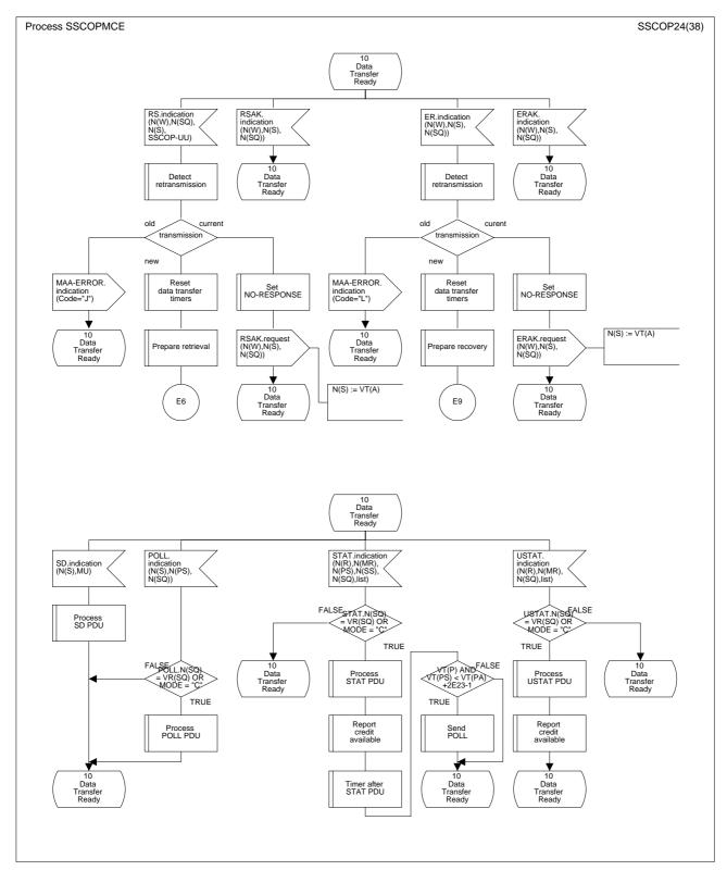
Figure 22/Q.2111 – SDL diagram of the multilink SSCOPMCE protocol entity (sheet 24 of 38)
