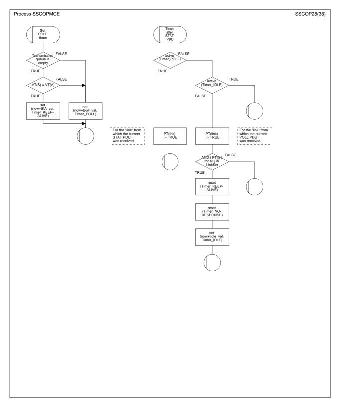
Figure 22/Q.2111 – SDL diagram of the multilink SSCOPMCE protocol entity (sheet 28 of 38)
