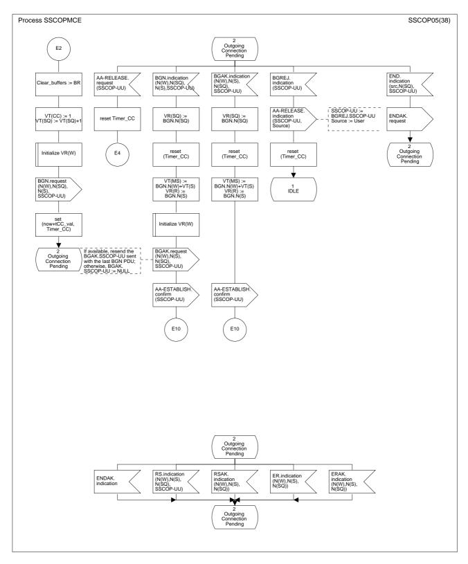
Figure 22/Q.2111 – SDL diagram of the multilink SSCOPMCE protocol entity (sheet 5 of 38)
