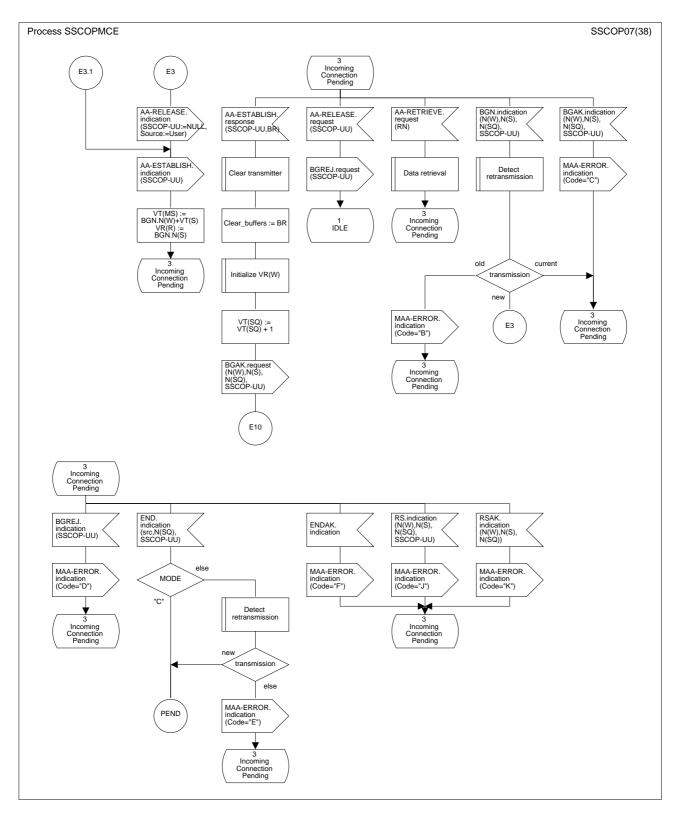
Figure 22/Q.2111 – SDL diagram of the multilink SSCOPMCE protocol entity (sheet 7 of 38)
