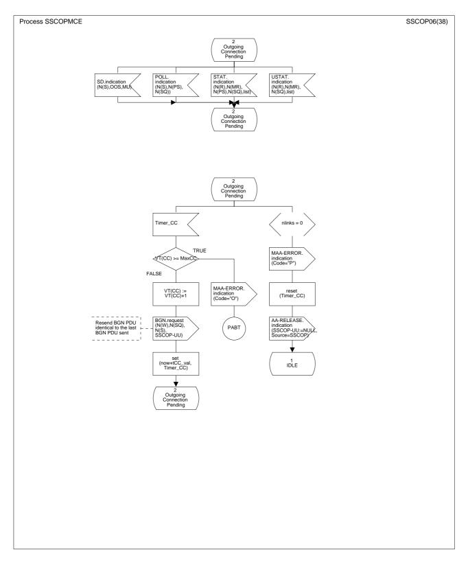
Figure 22/Q.2111 – SDL diagram of the multilink SSCOPMCE protocol entity (sheet 6 of 38)
