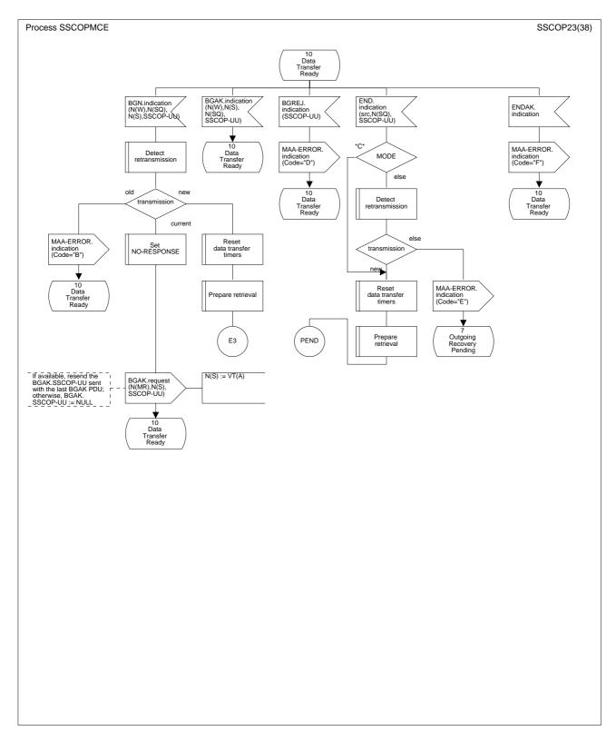
Figure 22/Q.2111 – SDL diagram of the multilink SSCOPMCE protocol entity (sheet 23 of 38)
