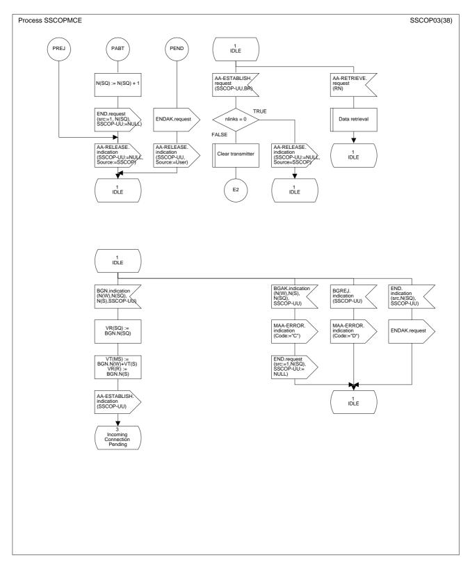
Figure 22/Q.2111 – SDL diagram of the multilink SSCOPMCE protocol entity (sheet 3 of 38)
