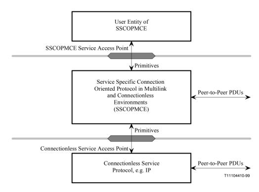
Figure 3/Q.2111 – SSCOPMCE in a connectionless environment
