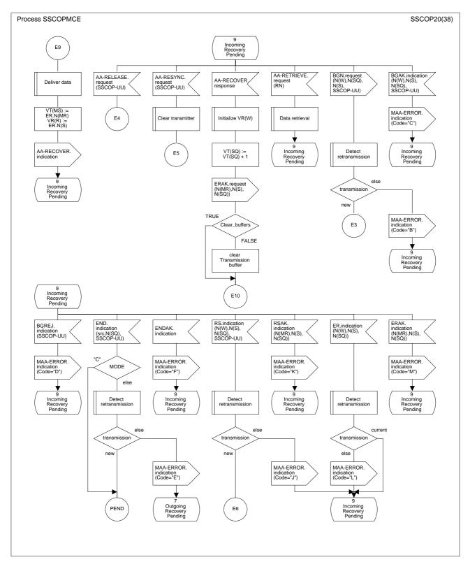
Figure 22/Q.2111 – SDL diagram of the multilink SSCOPMCE protocol entity (sheet 20 of 38)
