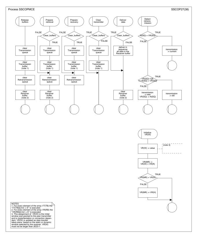
Figure 22/Q.2111 – SDL diagram of the multilink SSCOPMCE protocol entity (sheet 27 of 38)
