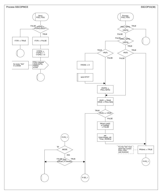
Figure 22/Q.2111 – SDL diagram of the multilink SSCOPMCE protocol entity (sheet 33 of 38)
