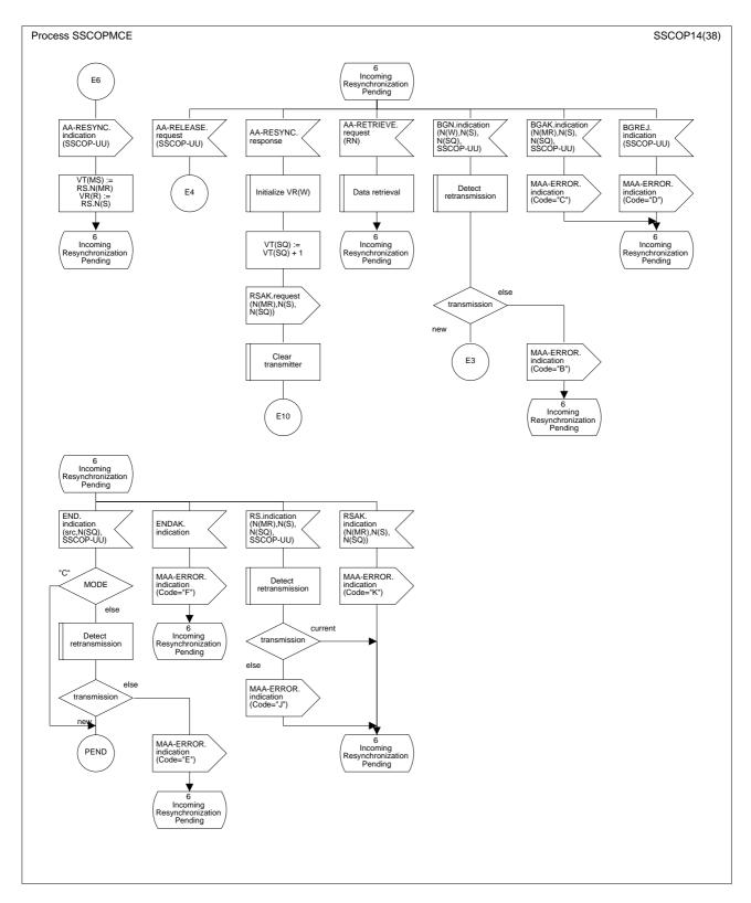
Figure 22/Q.2111 – SDL diagram of the multilink SSCOPMCE protocol entity (sheet 14 of 38)
