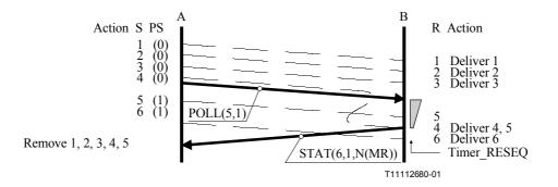
Figure II.17/Q.2111 – Acknowledgment of SD PDUs received after a POLL PDU but before Timer\_RESEQ expires
