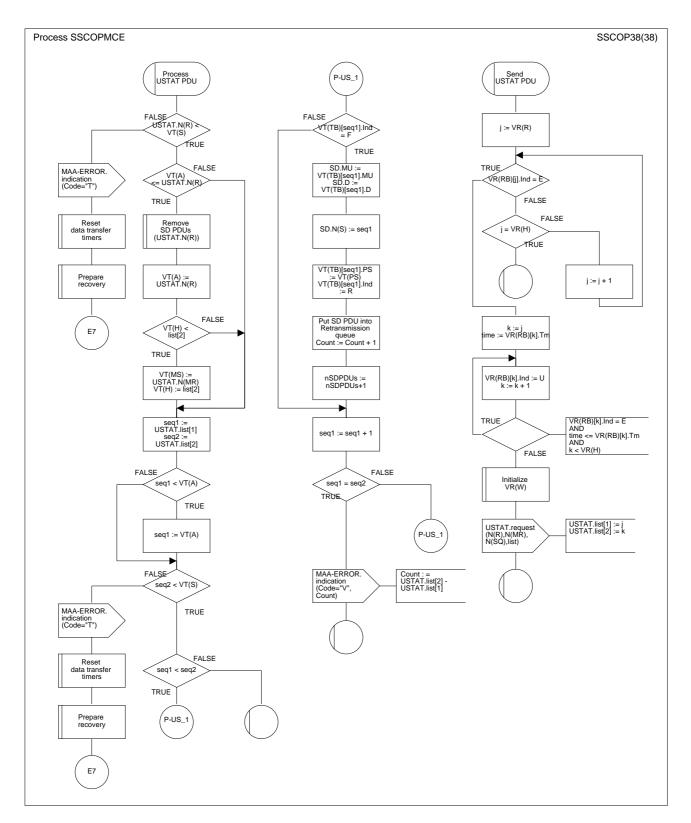
Figure 22/Q.2111 – SDL diagram of the multilink SSCOPMCE protocol entity (sheet 38 of 38)
