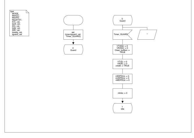
Figure 22/Q.2111 – SDL diagram of the multilink SSCOPMCE protocol entity (sheet 2 of 38)
