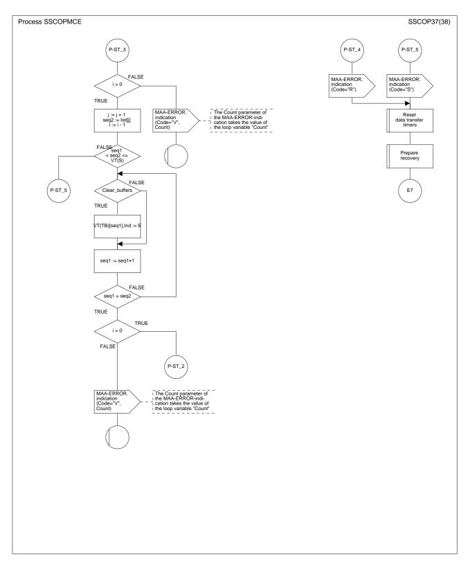
Figure 22/Q.2111 – SDL diagram of the multilink SSCOPMCE protocol entity (sheet 37 of 38)
