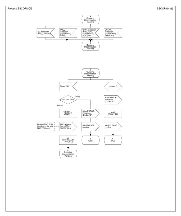
Figure 22/Q.2111 – SDL diagram of the multilink SSCOPMCE protocol entity (sheet 10 of 38)
