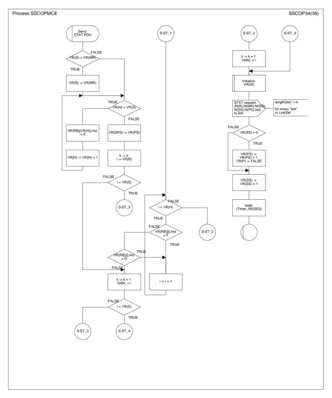
Figure 22/Q.2111 – SDL diagram of the multilink SSCOPMCE protocol entity (sheet 34 of 38)
