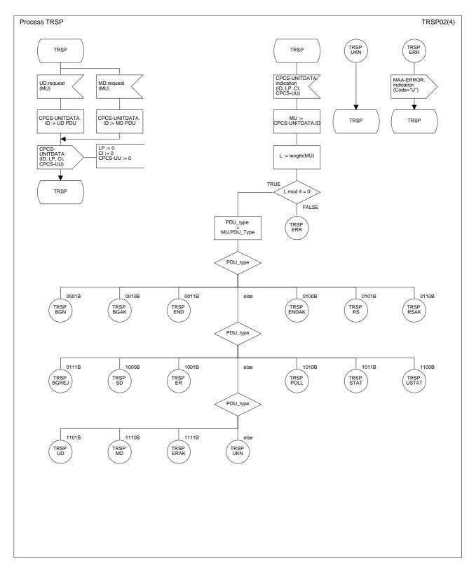
Figure B.1/Q.2111 – SDL diagram of the ancillary process TRSP (sheet 2 of 4)
