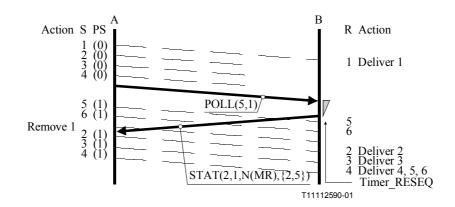
Figure II.8/Q.2111 – Error recovery via STAT PDU of the last transmitted SD PDUs
