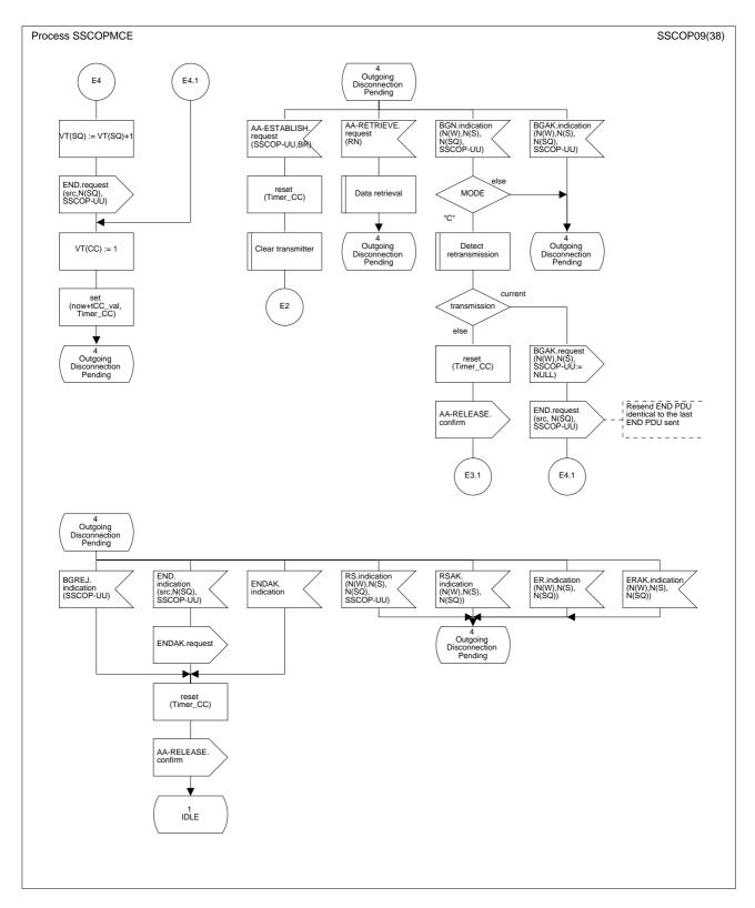
Figure 22/Q.2111 – SDL diagram of the multilink SSCOPMCE protocol entity (sheet 9 of 38)
