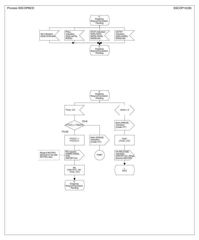
Figure 22/Q.2111 – SDL diagram of the multilink SSCOPMCE protocol entity (sheet 13 of 38)
