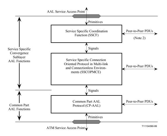
NOTE 1 – The figure represents the allocation of functions and is not extended to illustrate sublayers as definided by OSI modelling principles. NOTE 2 – A particular SSCF may include a protocol for the exchange of PDUs.
