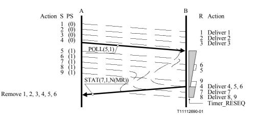
Figure II.18/Q.2111 – Acknowledgment of SD PDUs received after a POLL PDU with missing sequence of SD PDUs
