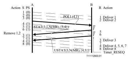
Figure II.9/Q.2111 – Error recovery via STAT and USTAT PDU of the last transmitted SD PDUs
