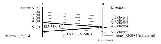
Figure II.5/Q.2111 – Operation in the error-free case
