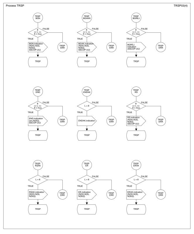
Figure B.1/Q.2111 – SDL diagram of the ancillary process TRSP (sheet 3 of 4)
