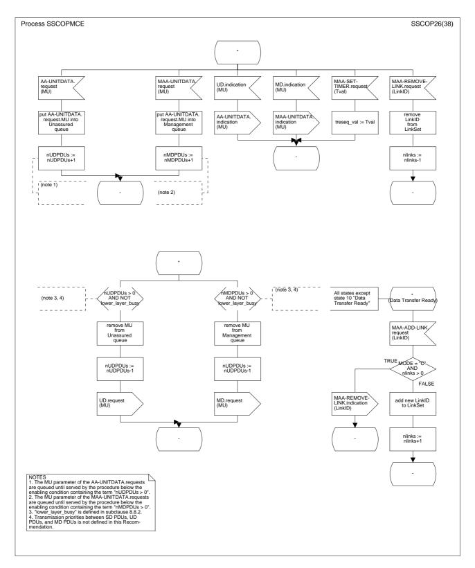
Figure 22/Q.2111 – SDL diagram of the multilink SSCOPMCE protocol entity (sheet 26 of 38)
