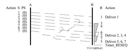
Figure II.16/Q.2111 – Recovery of out-of-sequence receipt of several SD PDUs with Timer\_RESEQ
