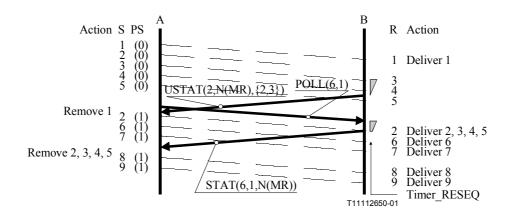
Figure II.14/Q.2111 – Error recovery of two missing SD sequences via STAT and USTAT PDUs (last SD PDU not missing)
