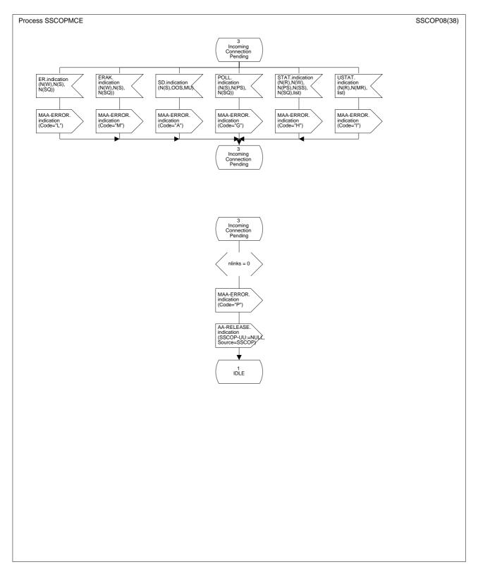
Figure 22/Q.2111 – SDL diagram of the multilink SSCOPMCE protocol entity (sheet 8 of 38)
