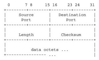
Figure C.4/Q.2111 – UDP header format
