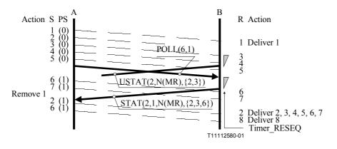
Figure II.7/Q.2111 – Error recovery via STAT PDU
