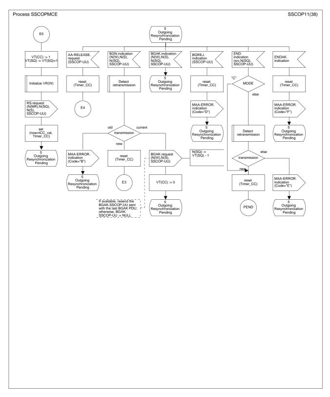
Figure 22/Q.2111 – SDL diagram of the multilink SSCOPMCE protocol entity (sheet 11 of 38)
