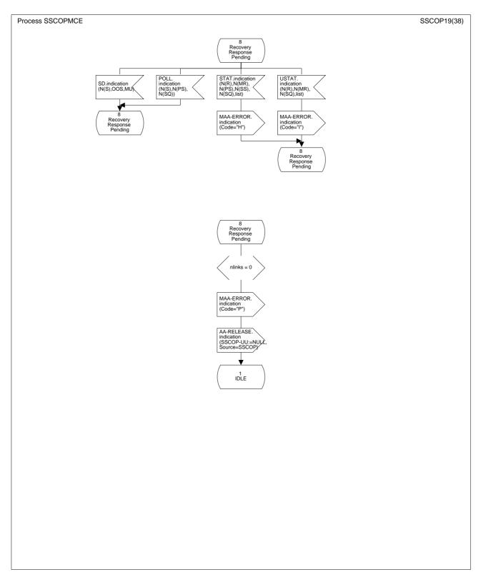
Figure 22/Q.2111 – SDL diagram of the multilink SSCOPMCE protocol entity (sheet 19 of 38)
