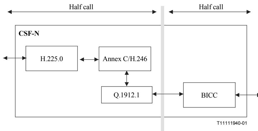
Figure 2/Q.1912.3 – Functional description of the interworking configuration
