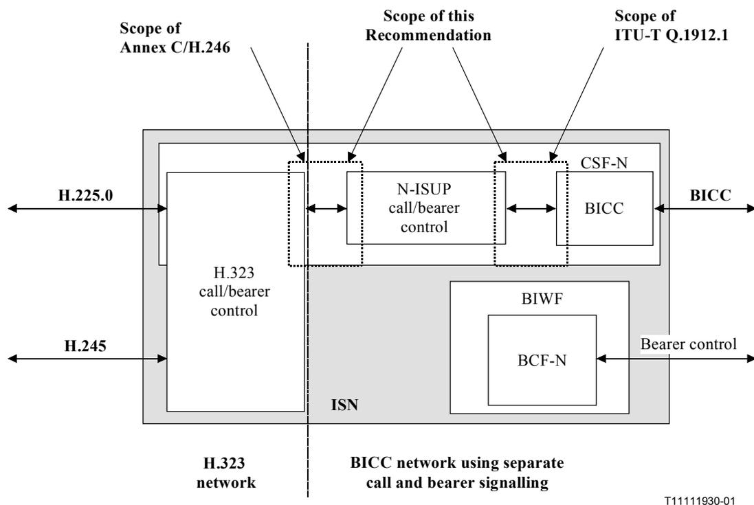
**Figure 1/Q.1912.3 – Scope of this Recommendation for BICC/H.225.0 interworking**
