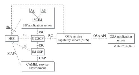
Figure 6-11 – Functional architecture for the provision of service in the IMS
