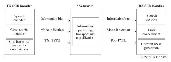
Figure 10.5.27-1 – Block diagram of one link SCR operation
