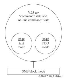
Figure 10.6.4-1 – Block, text and PDU modes
