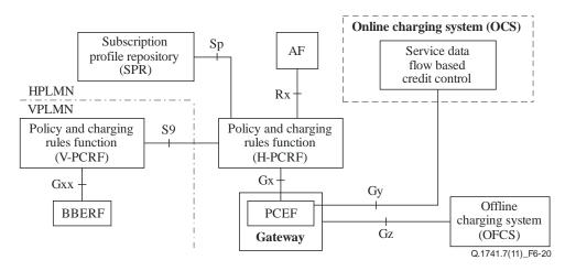
Figure 6-20 – PCC architecture (roaming with home routed access)
