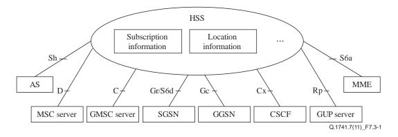
Figure 7.3-1 – Example of a generic HSS structure and basic interfaces
