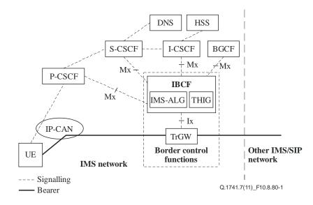
Figure 10.8.80-1 – Reference model for IMS Border Control Functions
