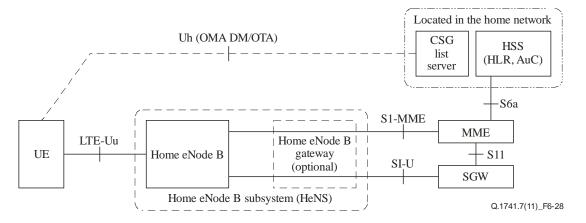
Figure 6-28 – Configuration of PLMN supporting Home eNodeB Subsystem
