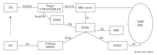
Figure 6-23 – SRVCC architecture for UTRAN (HSPA) to 3GPP UTRAN/GERAN with Gn based SGSN
