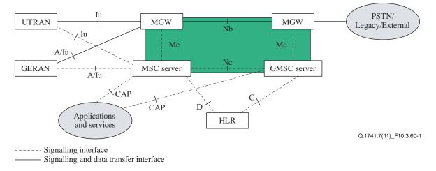
Figure 10.3.60-1 – CS core network logical architecture
