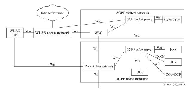
Figure 6-16 – Configuration of a 3GPP/WLAN interworking function
