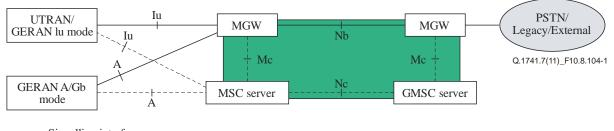
Figure 10.8.104-1 – CS core network logical architecture
