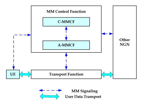
**Figure 7-2 – Functional architecture of MMCF in NGN**
