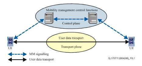
Figure 6-1 – MM control functionality
