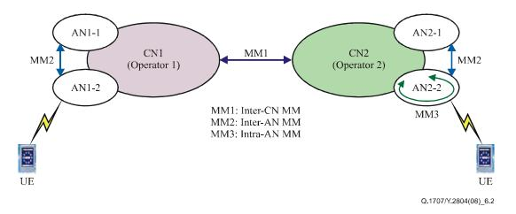
Figure 6-2 – Types of MM in NGN networks
