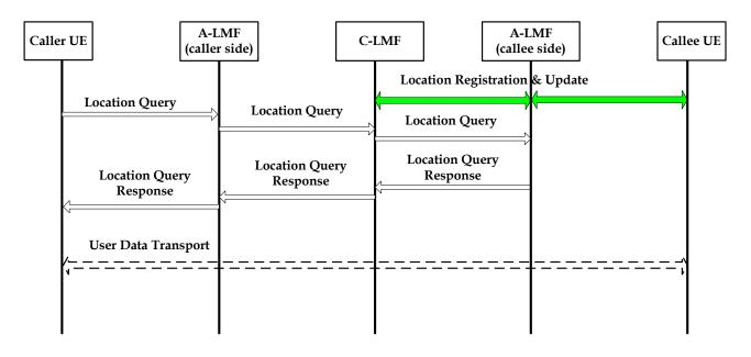
Figure 8-4 – Location query without session set-up signalling in the non-roaming case
