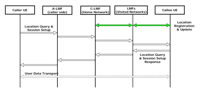
Figure 8-7 – Location query with session set-up signalling for the roaming case
