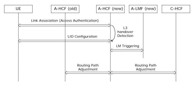
Figure 8-9 gives an example of the high-level information flow for handover execution.
