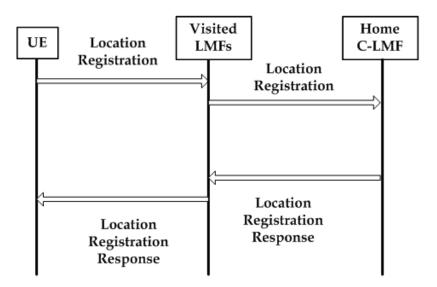
Figure 8-2 – Location registration for the roaming case
