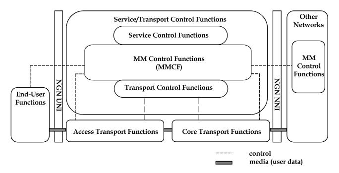
Figure 7-7 – Relationship between MMCF and NGN-FRA functions
