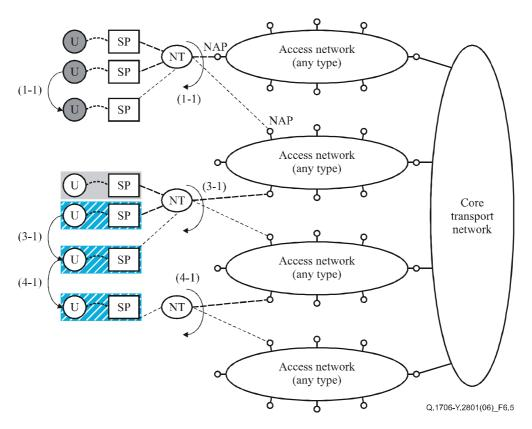
Figure 6-5/Q.1706/Y.2801 – Single NT with multiple ANs
