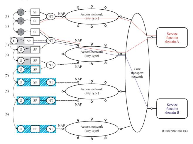
Figure 6-4/Q.1706/Y.2801 – Mobility scenarios according to the changes of endpoint
