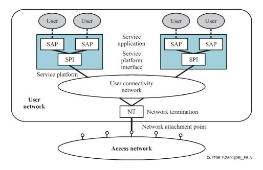
Figure 6-3/Q.1706/Y.2801 – User network configuration
