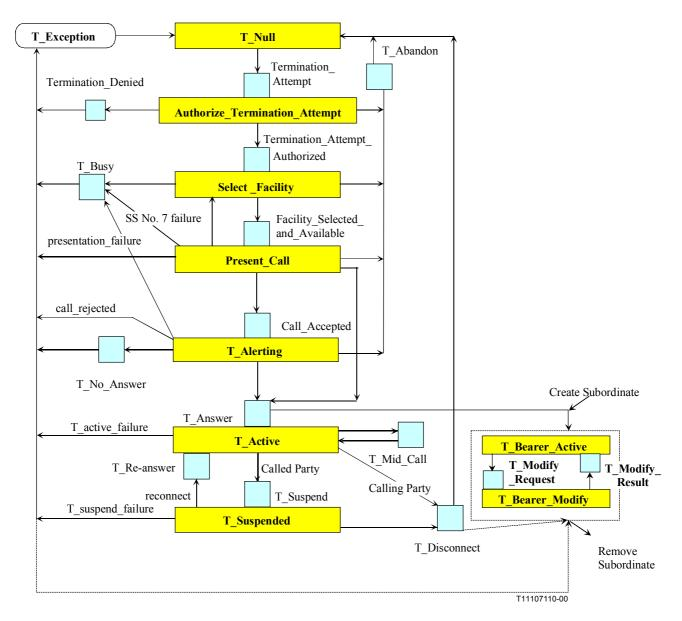
Figure 2/Q.1237 – Terminating BCSM for ITU-T Q.1237: Basic set of transitions
