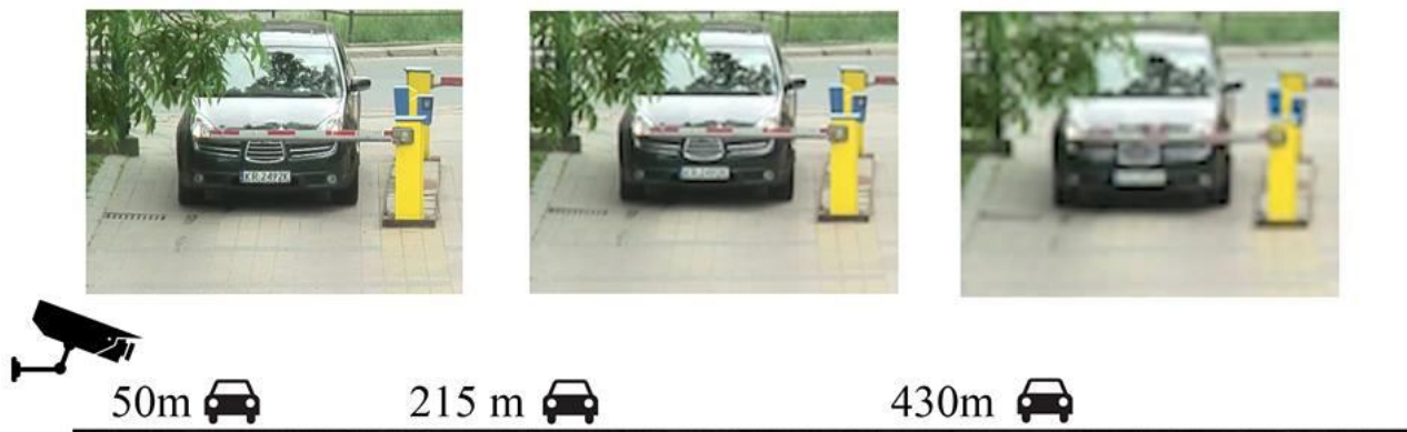
Figure 1 – DC in testing methods for various distances between camera and object
