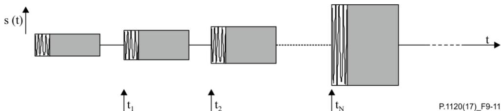
**Figure 9-11 – Test signal to determine the minimum activation level and the built-up time**
