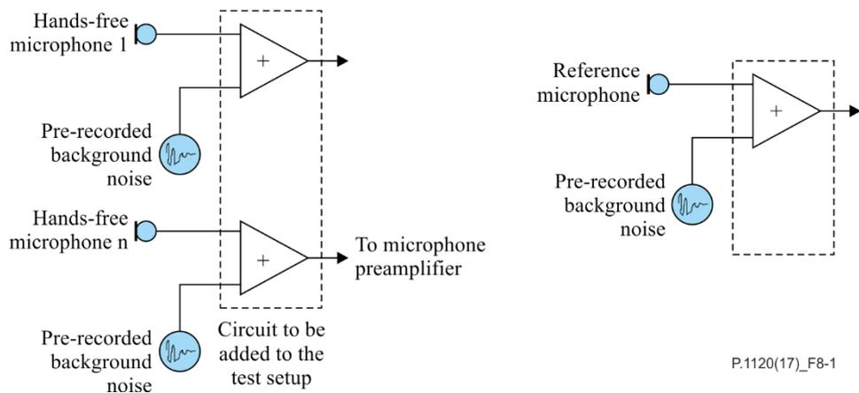
**Figure 8-1 – Set-up for insertion of the pre-recorded background noise signal at the hands-free microphone(s) and the reference microphone**
