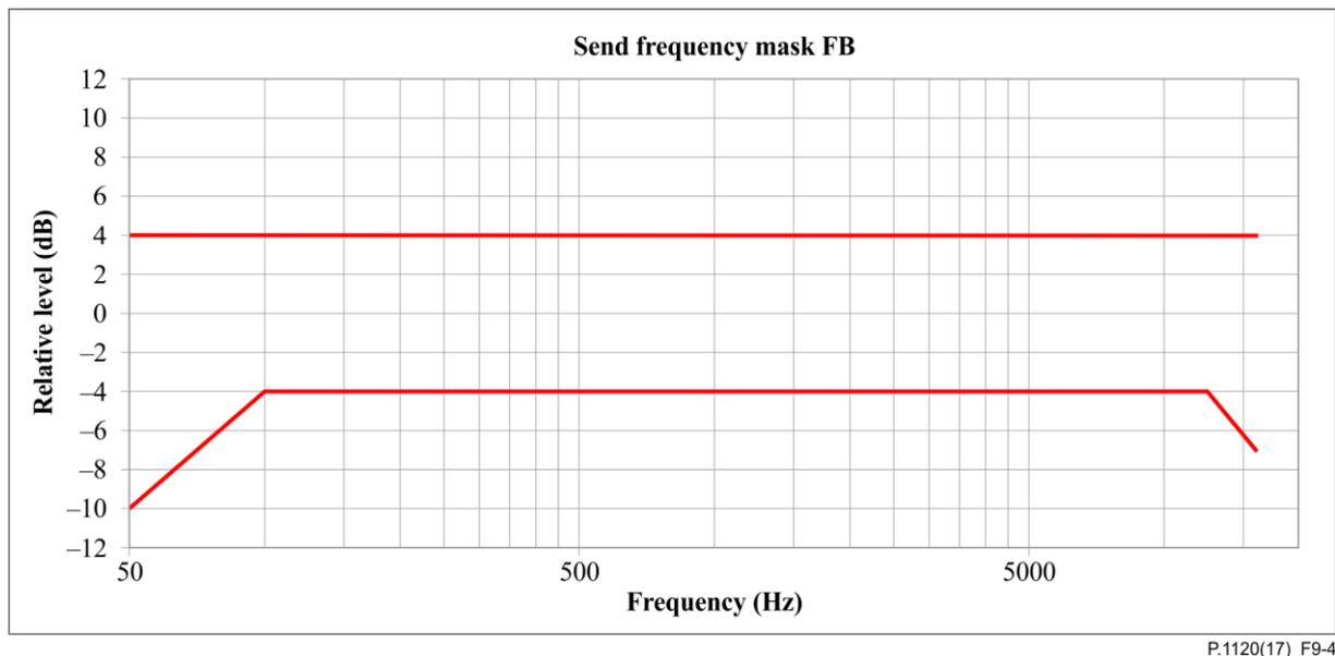
**Figure 9-4 – Tolerance mask for the FB send sensitivity frequency response
