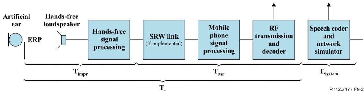
**Figure 9-2 – Different blocks contributing to the delay in receive direction**
