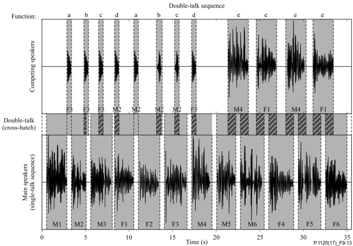
**Figure 9-13 – Double talk test sequence with overlapping speech sequences in send and receive directions**
