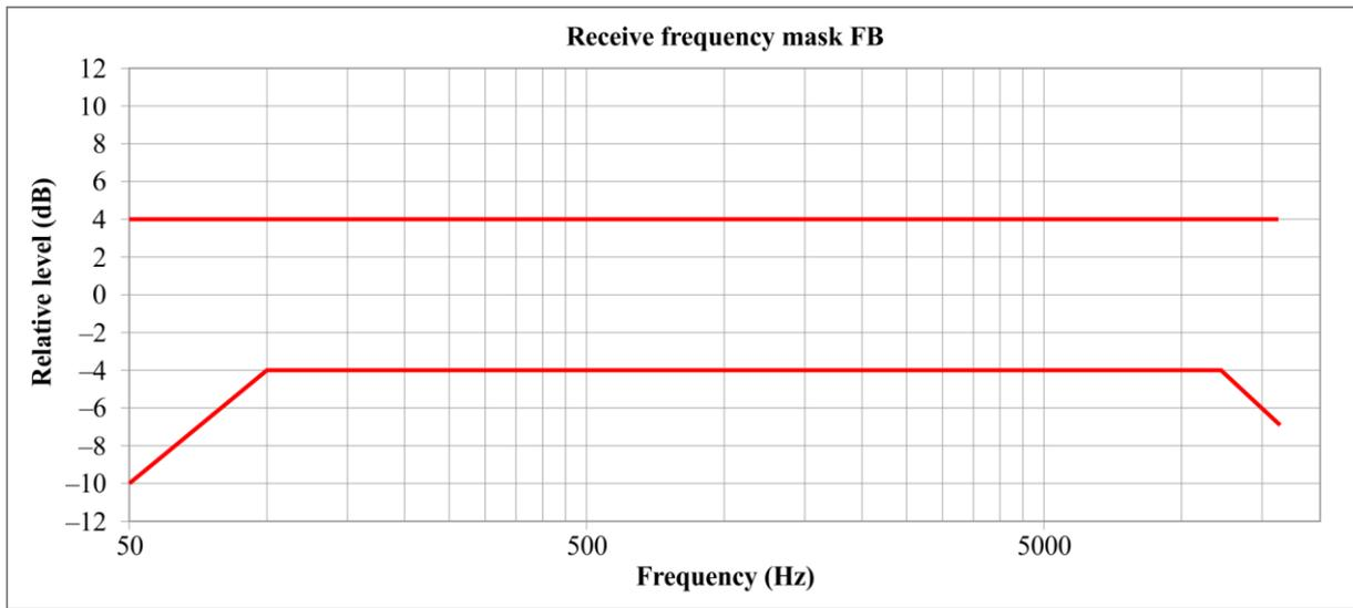
**Figure 9-6 – Tolerance mask for the FB receive sensitivity frequency response (Figure is informative)**
