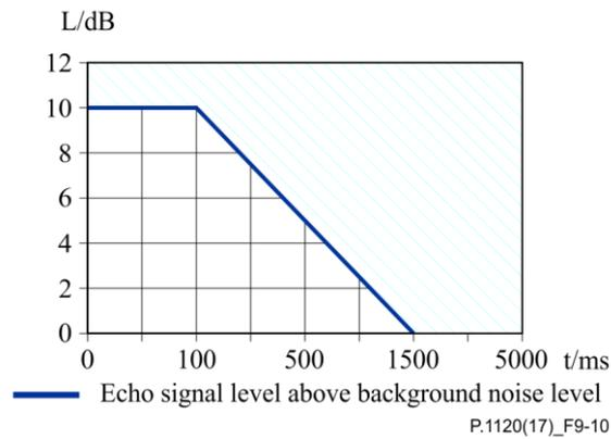
**Figure 9-10 – Initial convergence with background noise, requirement on echo signal level vs time**
