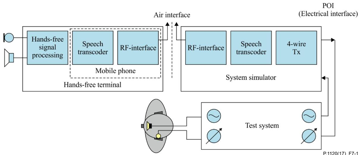
**Figure 7-1 – Test arrangement for hands-free terminal**
