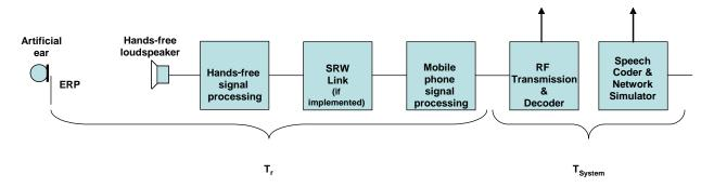
Figure 11-2 – Different blocks contributing to the delay in receiving
