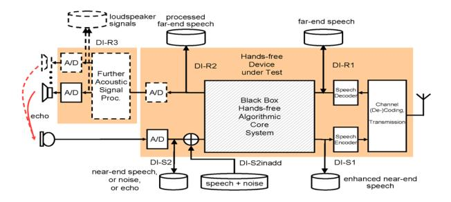
Figure 8-1 – Digital interfaces for the HF system
