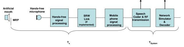
Figure 11-1 – Different blocks contributing to the delay in sending
