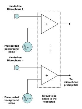
NOTE – Structure-borne noise is also covered with this arrangement, which is part of the microphone recording.
