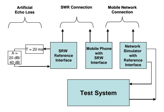
Figure 12-3 – Test setup with artificial echo loss
