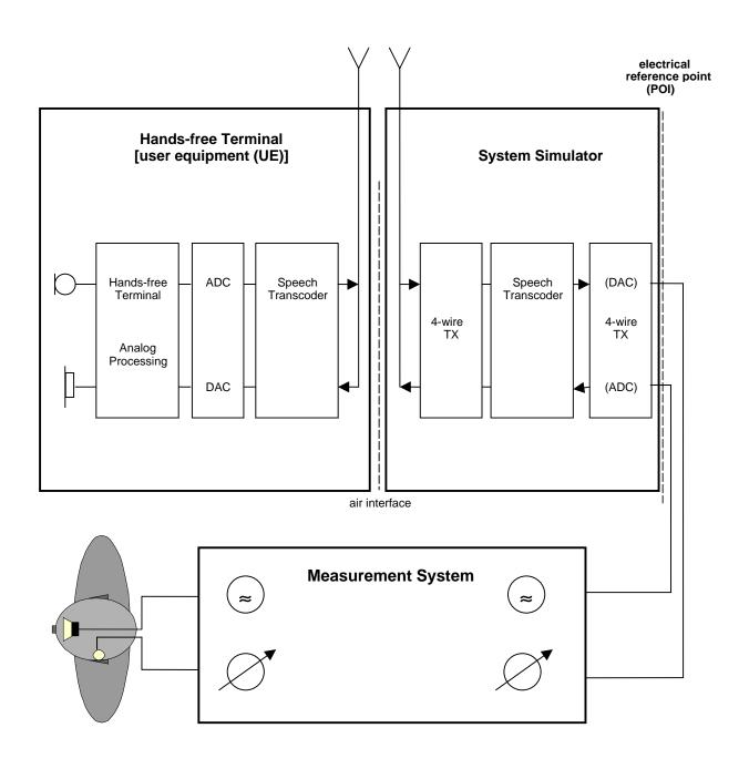
Figure 7-1 – Test arrangement for hands-free terminals
