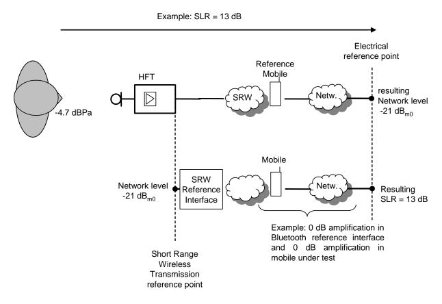
Figure 12-2 – Calibration of the short-range wireless transmission reference interface
