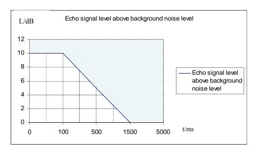
Figure 11-4 – Initial convergence with background noise, requirement on echo signal level versus time
