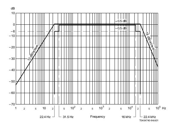
$FIGURE \ \ 1/O.41$  Frequency response characteristics for unweighted measurements
