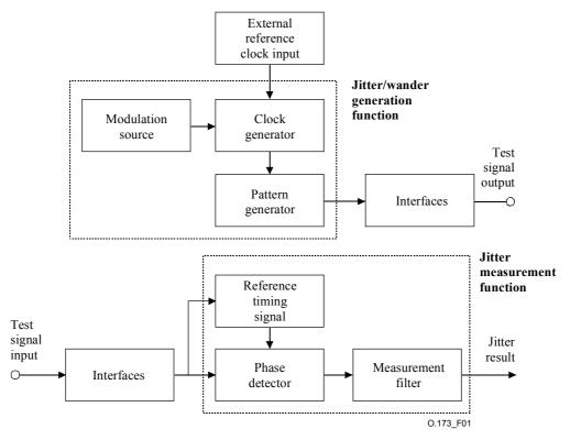
Figure 1/O.173 – Functional block diagram for jitter test set
