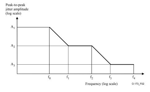
Figure 2/0.173 – Generated jitter amplitude versus jitter frequency
