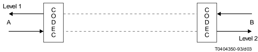
FIGURE 3/N.86 Designations for levels and ends for audio tests
