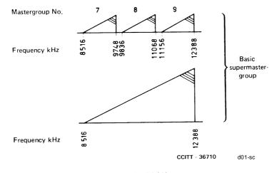
FIGURE 1/M.350 Numbering of mastergroup within a supermastergroup
