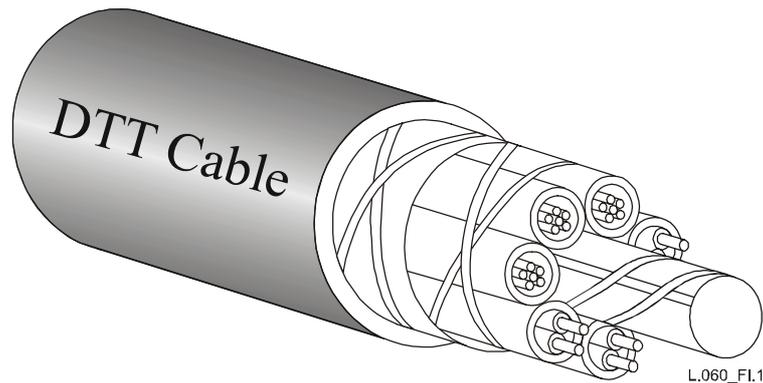
**Figure I.1/L.60 – The 3-dimensional sketch map of the optical fibre/copper hybrid cable**
