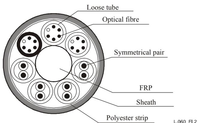
**Figure I.2/L.60 – Construction of an optical fibre/symmetrical pair hybrid cable**
