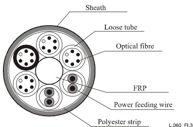
**Figure I.3/L.60 – Cross-section of optical fibre/stranded copper wire hybrid cable**
