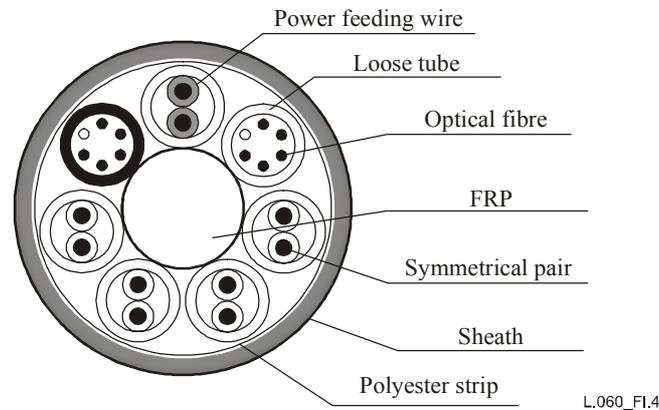
**Figure I.4/L.60 – Cross-section of optical fibre/symmetrical pair/stranded copper wire hybrid cable**
