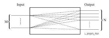
Figure 6-1 – MxN branching component (schematic)
