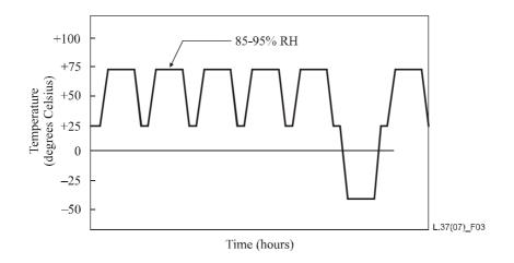
Figure 10-2 – Thermal profile of cyclic moisture resistance test
