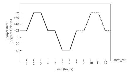
Figure 10-1 – Thermal profile of temperature humidity cycle test
