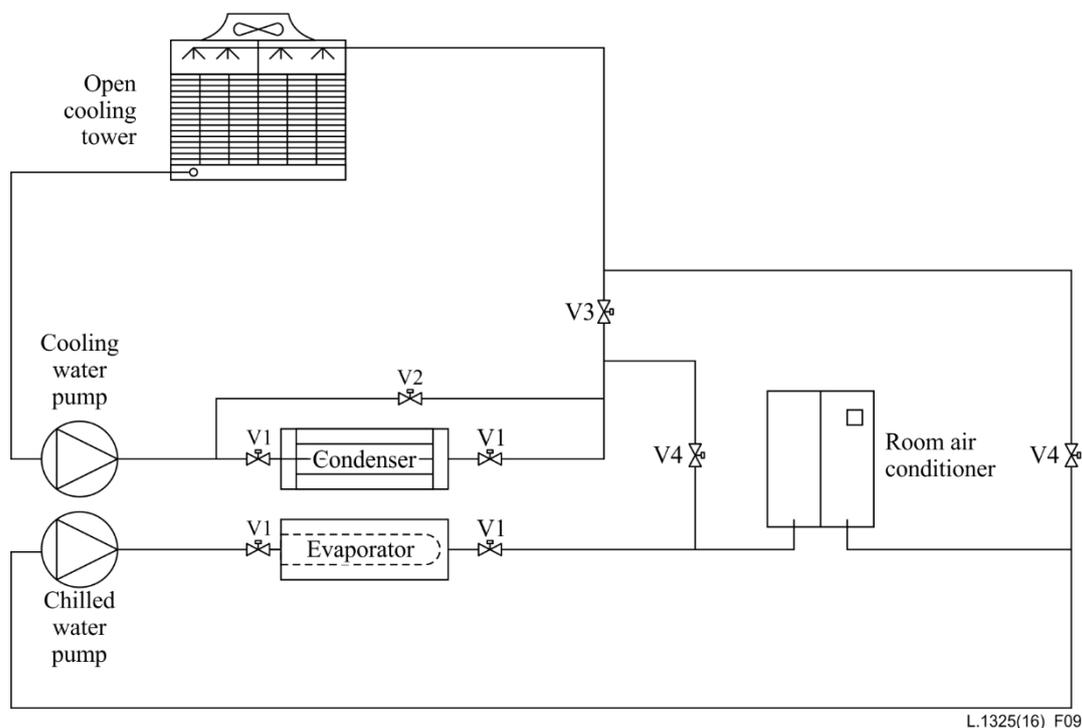
**Figure 9 – Closed cooling tower cooling system**
