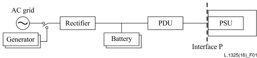
**Figure 1 – A power feeding system with backup solution including up to 400 VDC power feeding**
