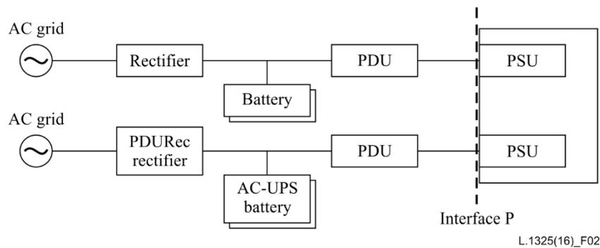
**Figure 2 – Dual AC supply system configuration for dual PSU ICT equipment**
