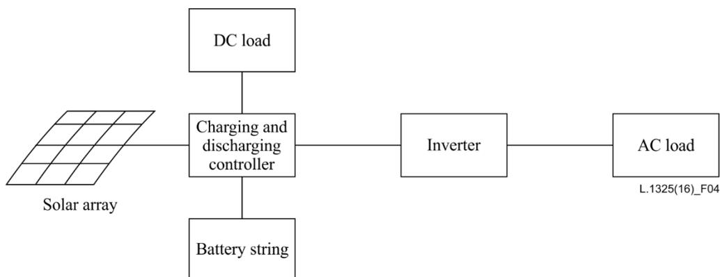
**Figure 4 – Off-grid solar power system**
