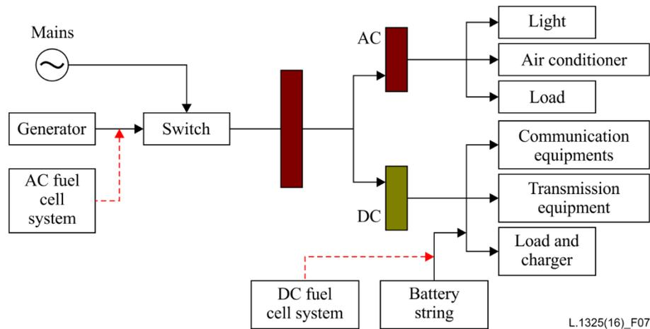
**Figure 7 – Hydrogen fuel cell-powered system DC power supply and AC power lines**
