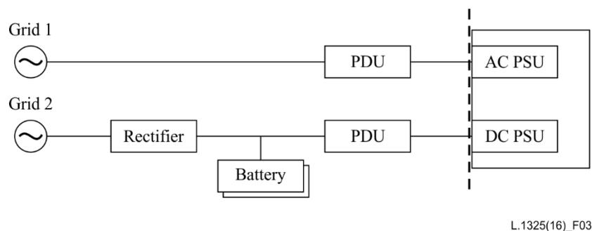
**Figure 3 – AC grid + HVDC power supply structure**
