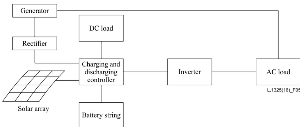
**Figure 5 – Solar and DG power system**
