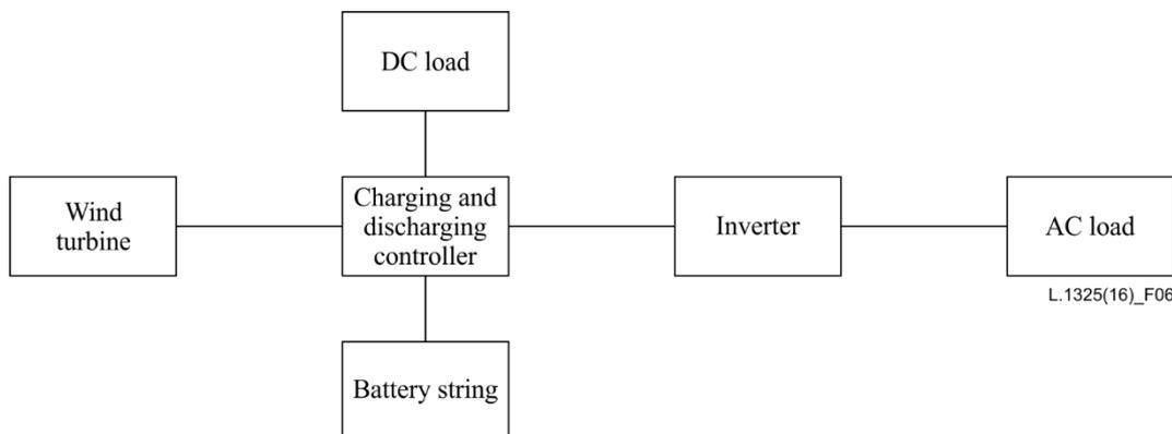
**Figure 6 – Off-grid wind power system structure**
